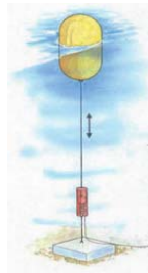
Figure 1 – Point Absorber Schematic.
