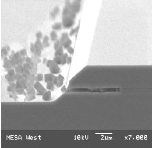
**Figure 7. Cross-sectional SEM of sample with release layer etched in BOE.**
