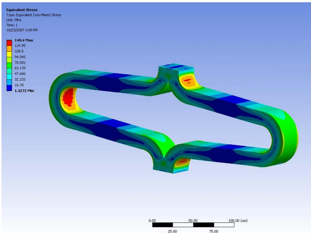
Figure 3. Stress distribution in spring when the elastic limit is reached (1.46 micron displacement).
