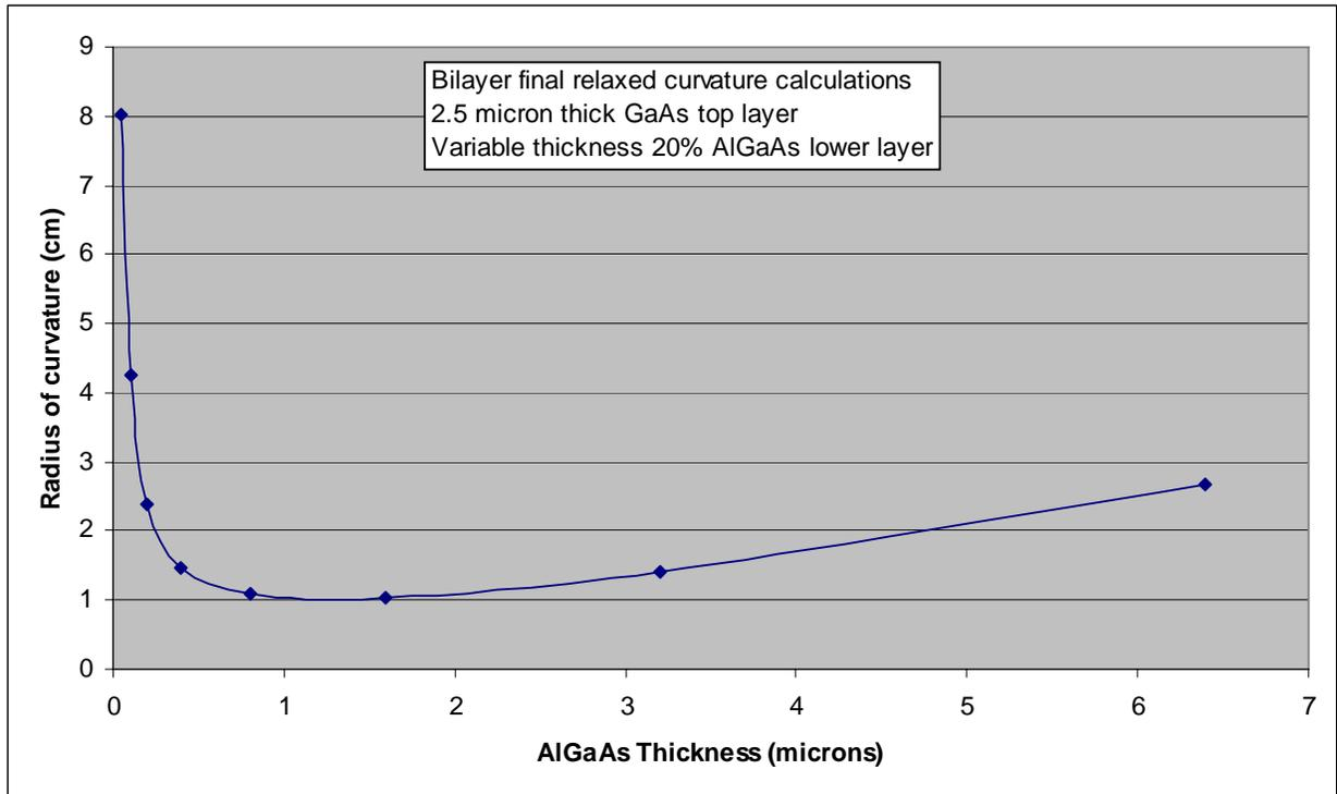
**Figure 4. Released cylinder final radius of curvature as a function of AlGaAs thickness in a 2.5 micron GaAs/20%AlGaAs bilayer.**
