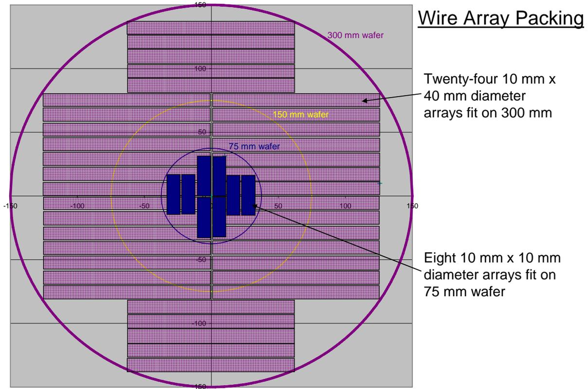
**Figure 18. Schematic of packing different size arrays on various wafer sizes.**
