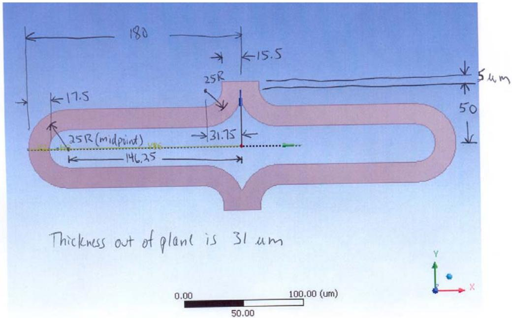
Figure 2. Layout of in-line spring to allow for anode-cathode displacements in Z.
