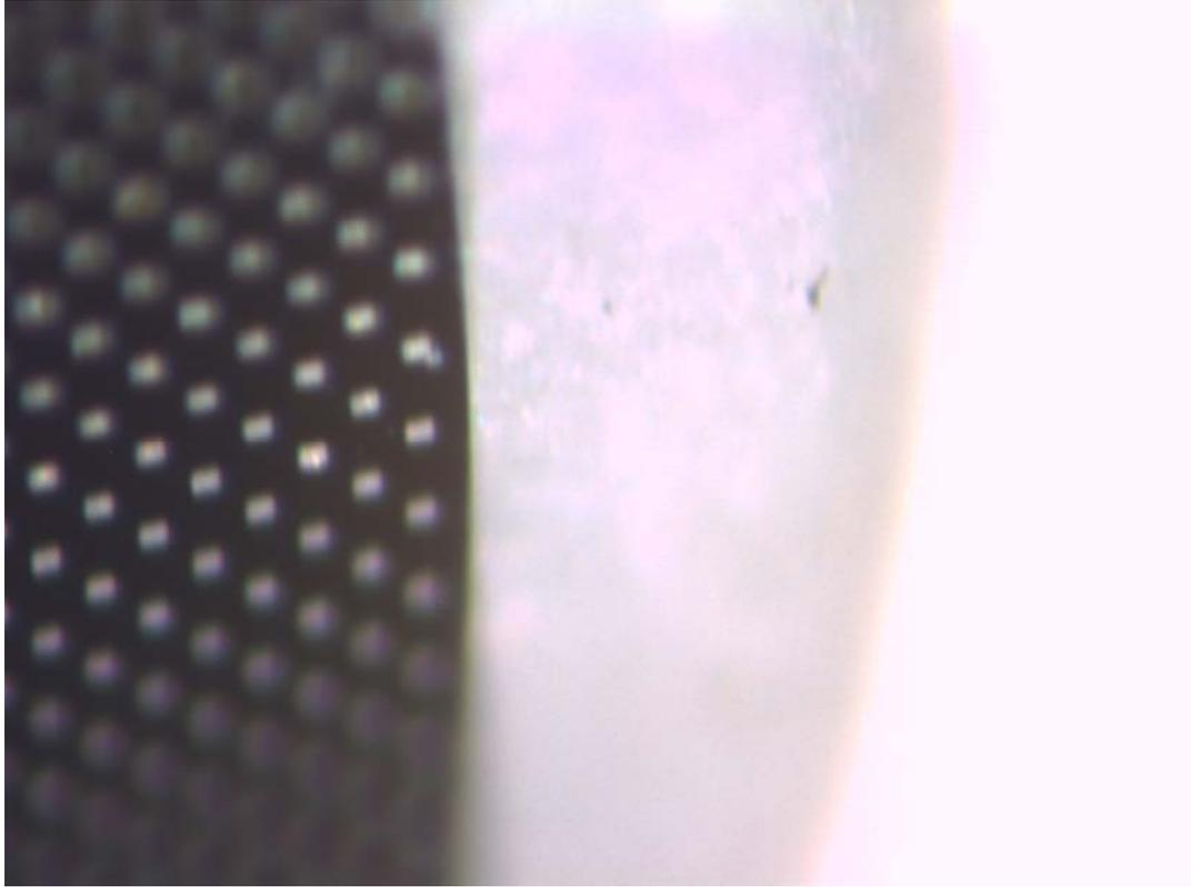
**Figure 6. Released GaAs/AlGaAs semiconductor support showing isolated release holes. The holes are on a 50 micron pitch.**
