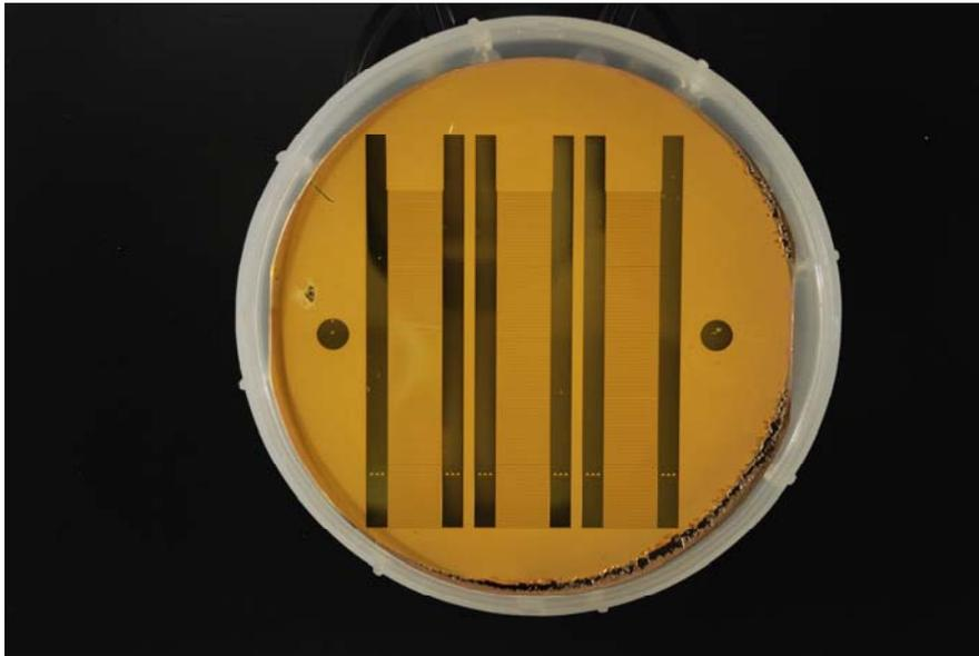
**Figure 12. Patterned and plated film showing zero resist defects in the pattern area. There are three wire arrays with 150, 62 micron wide wires plated to 15 microns. The arrays are designed to roll up into a diameter of 20 mm. The two circles are for plating contacts. The mustard-colored field is photoresist. The wafer diameter is 100mm.**
