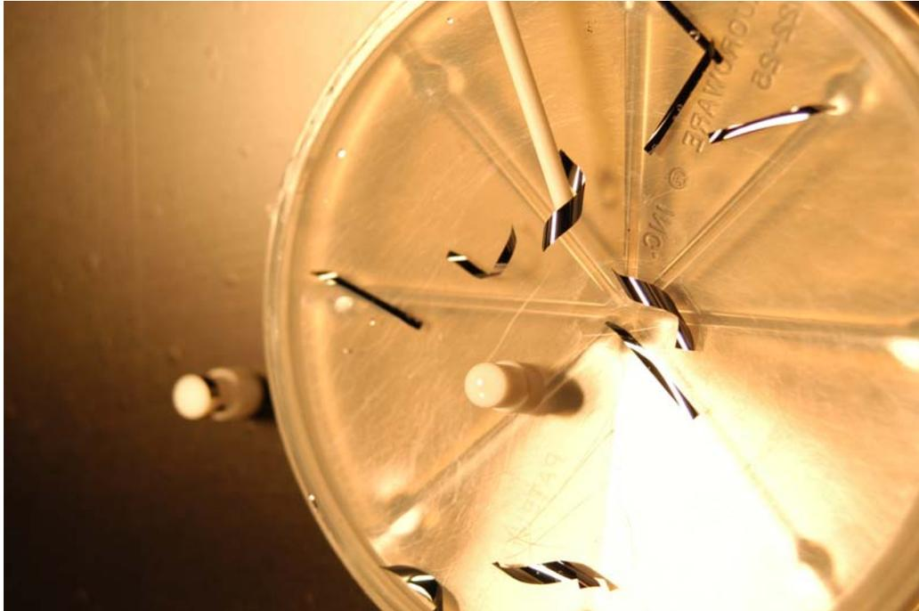
**Figure 9. A film electrostatically held on a macor rod (top of image).**
