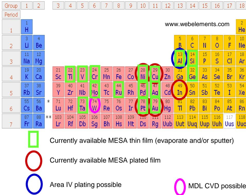
**Figure 19. Periodic table showing current metal deposition options.**
