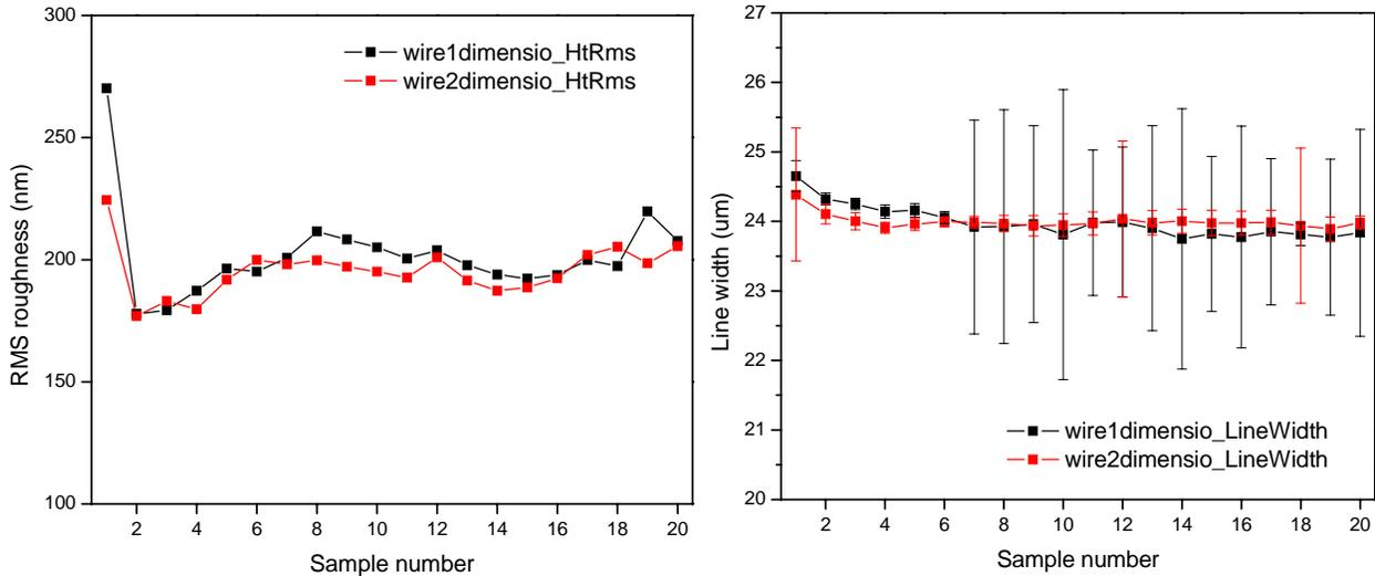
**Figure 15. Roughness (left) and line width (right). The large error bars in the right hand figure are an artifact of the data extraction; the small error bars are more representative.**
