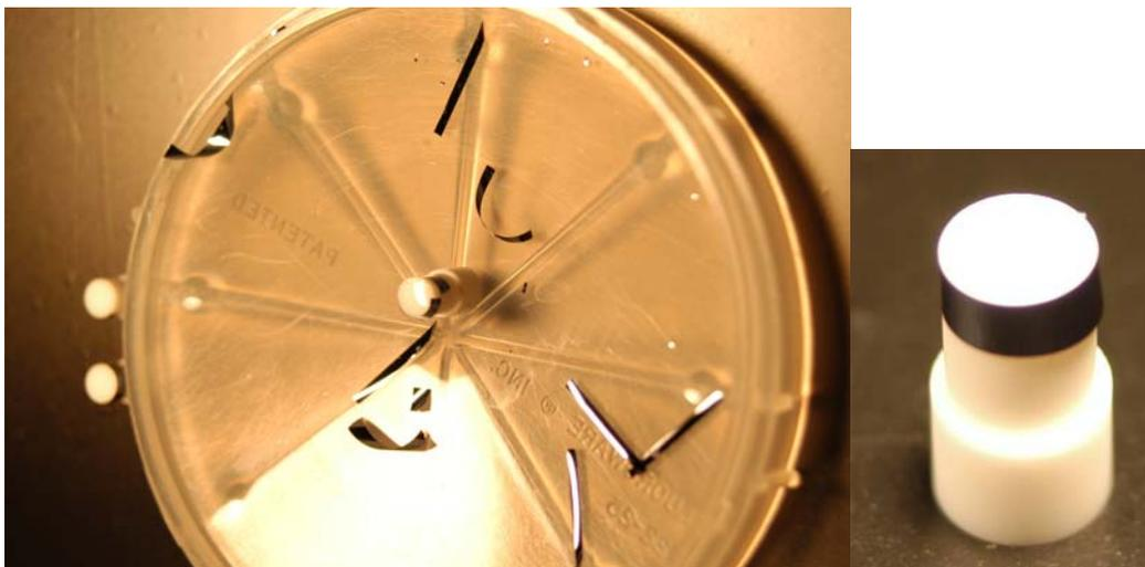
**Figure 10. Film placed onto moistened mandrel for manipulation to desired cylindrical shape. Right, after manipulation to form final cylinder shape.**
