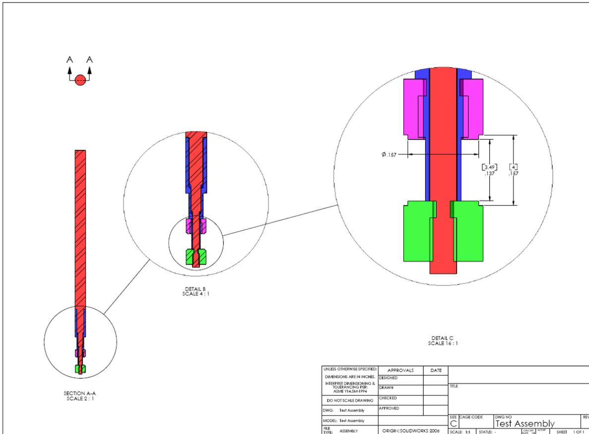
**Figure 16. First generation mounting hardware for 4mm diameter wire arrays. The anode (green) and cathode (pink) contacts are held in place by a threaded rod (red) and separated by a threaded spacer (blue). These last two items are removed after positioning the wire array in Z, with the wire array attached at the inset in the anode/cathode circumference.**
