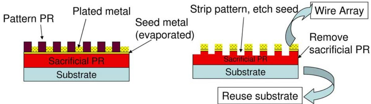
**Figure 13. Schematic of semiconductor-support-free wire array process flow.**
