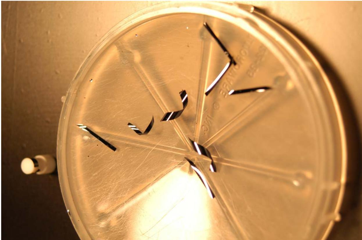
**Figure 8. Several released semiconductor supports. The unrolled length of each film is 12.56 mm, and the strip height is 1, 2, or 4 mm.**
