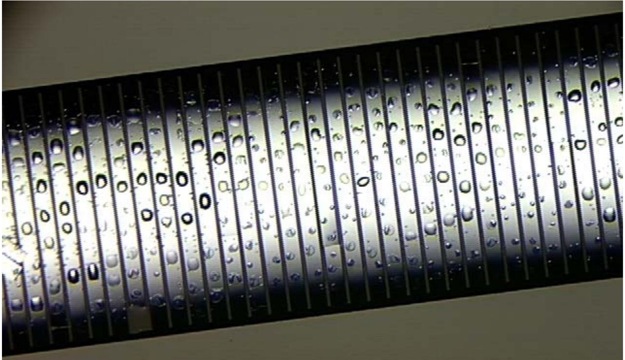
**Figure 5. Released 1-mm tall strip with slotted release holes. Etchant is 1:3 HF(49%):H<sub>2</sub>O. This etchant results in some blistering due to bubble formation. Note the slots lead to curvature in the short (axial) strip direction instead of the long (desired circumferential) direction.**
