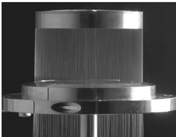
**Figure 1. A photograph of a 4-cm diameter tungsten wire array with 240, 7.5 micron diameter wires. From [4].**
