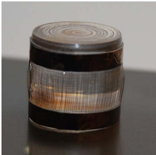
**Figure 17. Wire array mounted on a 2 cm polyethylene rod.**
