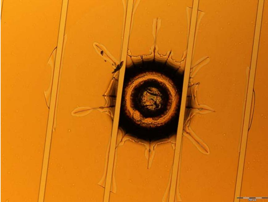
**Figure 11. Particle-and-stress defect in 35 micron thick AZ50XT resist. Note the cracking emanating from the pattern edges. The open lines are 30.6 microns wide.**
