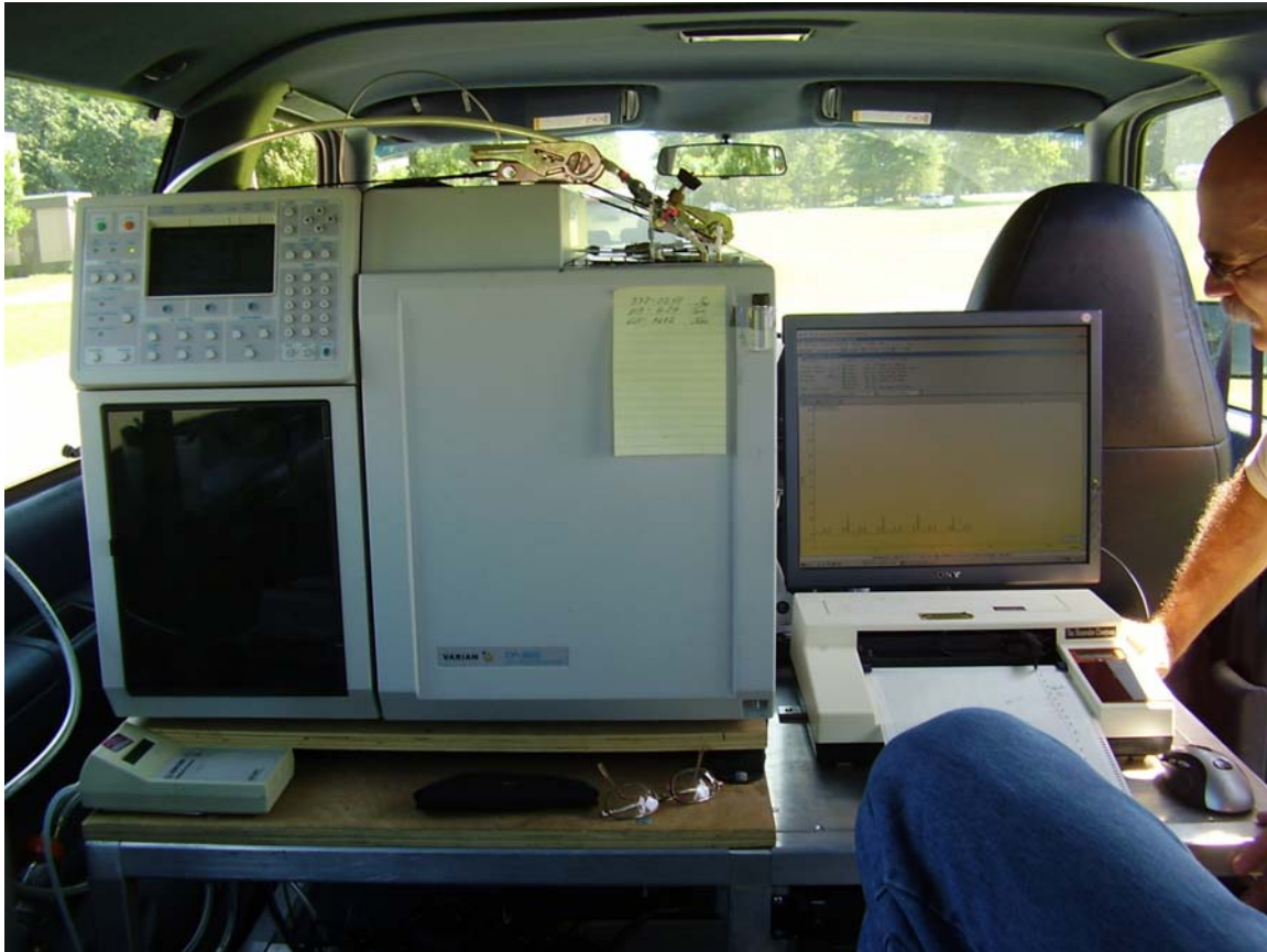
Figure 1 The Brookhaven Continuous Dual Trap Analyzer for Perfluorocarbon Tracer Detection
