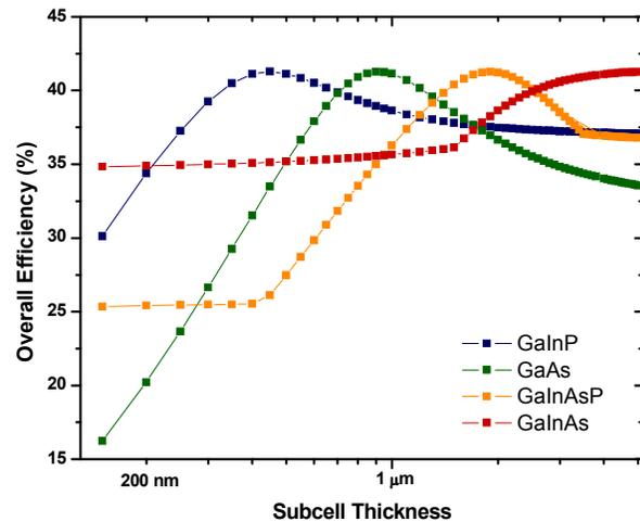
**Figure 13. Overall four junction efficiency as a function of subcell thickness, varying one cell thickness at a time.**
