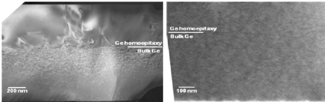
**Figure 2. Cross-sectional transmission electron microscopy images of Ge homoepitaxy on a Ge/Si template without damage removal (left) and with damage removal (right). The white line is at the interface of the substrate and the homoepitaxy.**
