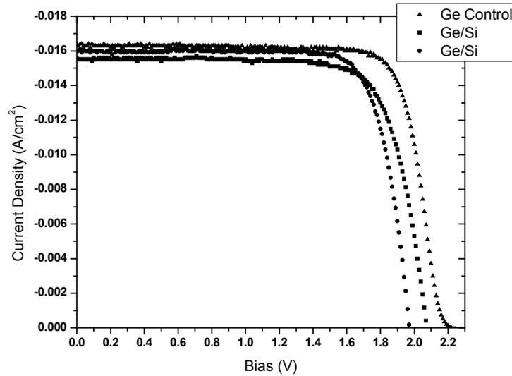
**Figure 4. Photovoltaic I-V curves for the GaInP/GaAs solar cells grown on Ge/Si epitaxial templates and on a bulk epi-ready Ge substrate**
