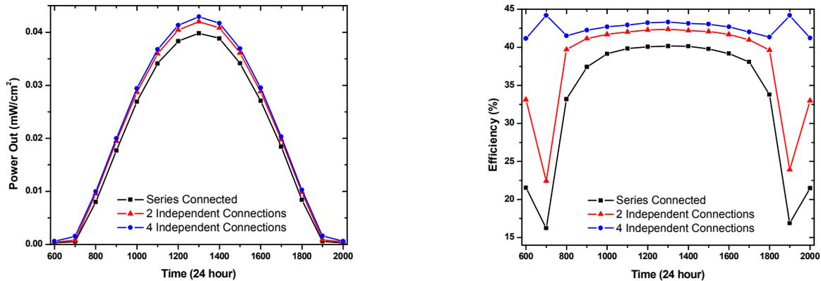
**Figure 15. Overall performance of the four junction cell as a function of the time of day for the three different electrical connections.**
