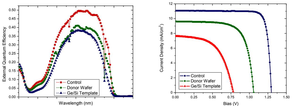
**Figure 6. External quantum efficiency and Light IV data for the first GaInP solar cell grown on Ge/Si templates.**
