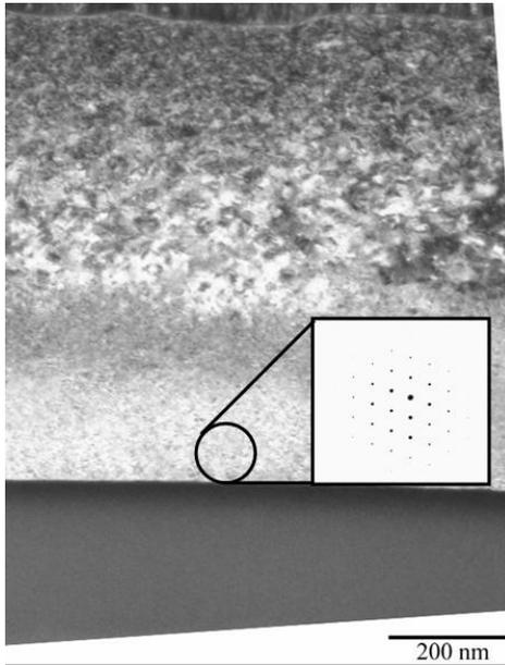
**Figure 11. Cross-sectional transmission electron microscope image of an InP/Si epitaxial template fabricated using InP implanted with 115 keV He<sup>+</sup> to a dose of  $1.0 \times 10^{17} \text{ cm}^{-2}$  showing the strain contrast caused by defects caused during ion implantation and (inset) selected-area diffraction image indicating that the InP adjacent to the bonded interface (within ~200 nm) is crystalline.**
