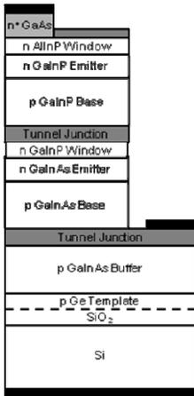
**Figure 3. Schematic cross-section of the dual junction solar cell grown and processed by Spectrolab. The bonded interface is shown by a dashed line.**
