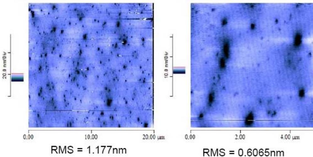
Figure 8. Representative AFM scans of the Ge surface after CMP
