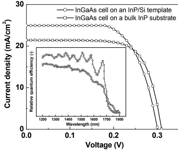
**Figure 12. Photovoltaic I-V curves and (inset) spectral responses for the InGaAs solar cells grown on the InP/Si epitaxial templates and on a commercial bulk epi-ready InP substrate. The I-V measurements were under a spectral portion truncated at 850 nm from 1-sun AM1.5G spectrum.**
