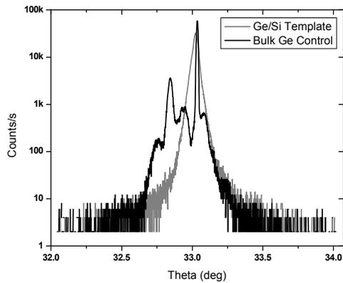
**Figure 5. High-resolution X-ray diffraction rocking curves for the GaInP/GaAs solar cells grown on Ge/Si epitaxial templates and on a bulk epi-ready Ge substrate.**
