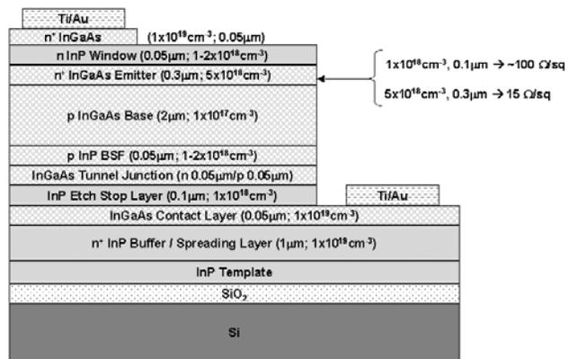
Figure 9. Schematic of InGaAs/InP/SiO<sub>2</sub>/Si cell
