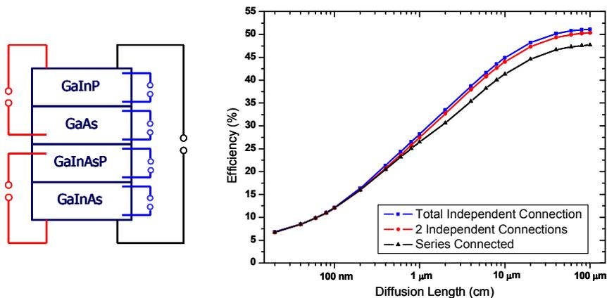
**Figure 14. Overall cell efficiency as a function of the diffusion length in all four subcells for 3 different electrical connections.**
