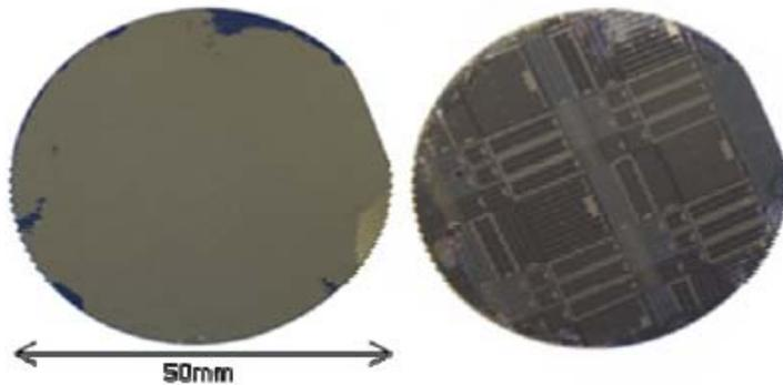
**Figure 1. Optical micrographs of a full 50mm Ge/Si template made with layer transfer and wafer bonding (left), and GaInP/GaAs solar cells grown on a Ge/Si template (right).**
