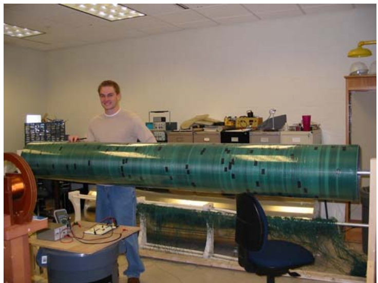
Fig. 2: The solenoid shielded chamber can provide extremely uniform static magnetic field with a magnetic field of up to 1.8 Gauss
