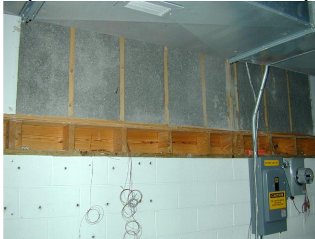
Figure 6. ORNL test wall containing PCM-enhanced cellulose insulation.
