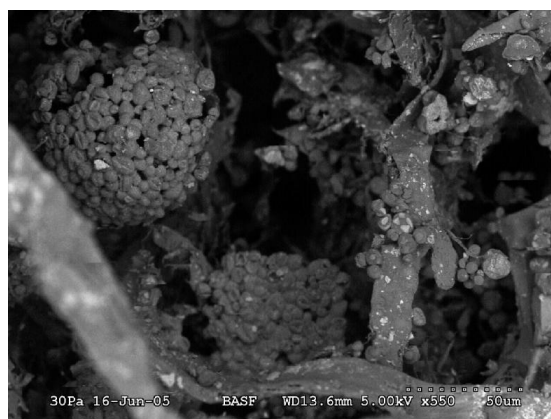
Cellulose with 30% PCM: clusters of PCM pellets are visible.
