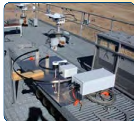
Two shadowbands rotate around the TCRSR sensor, located just inside the smaller shadowband. As they sequentially rotate about their axis, the downwelling irradiance is partially blocked, allowing irradiance variations across the solar aureole to be observed.
