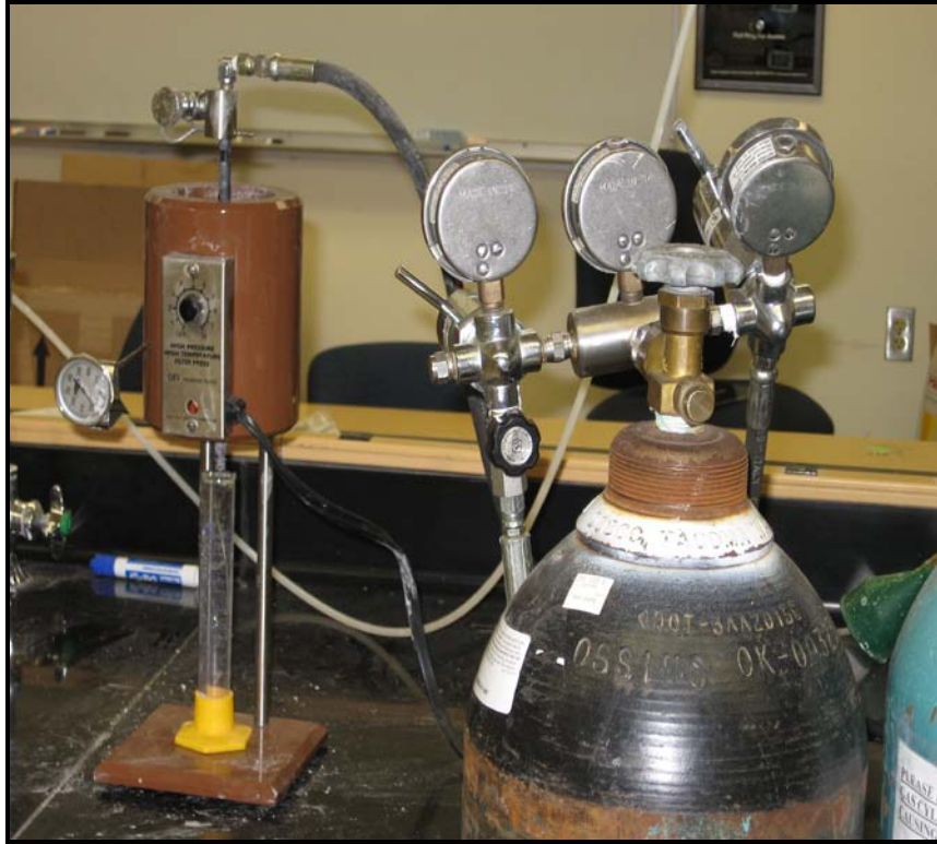
Figure 37: Fluid-Loss Measuring Apparatus at the University of Alaska Fairbanks
