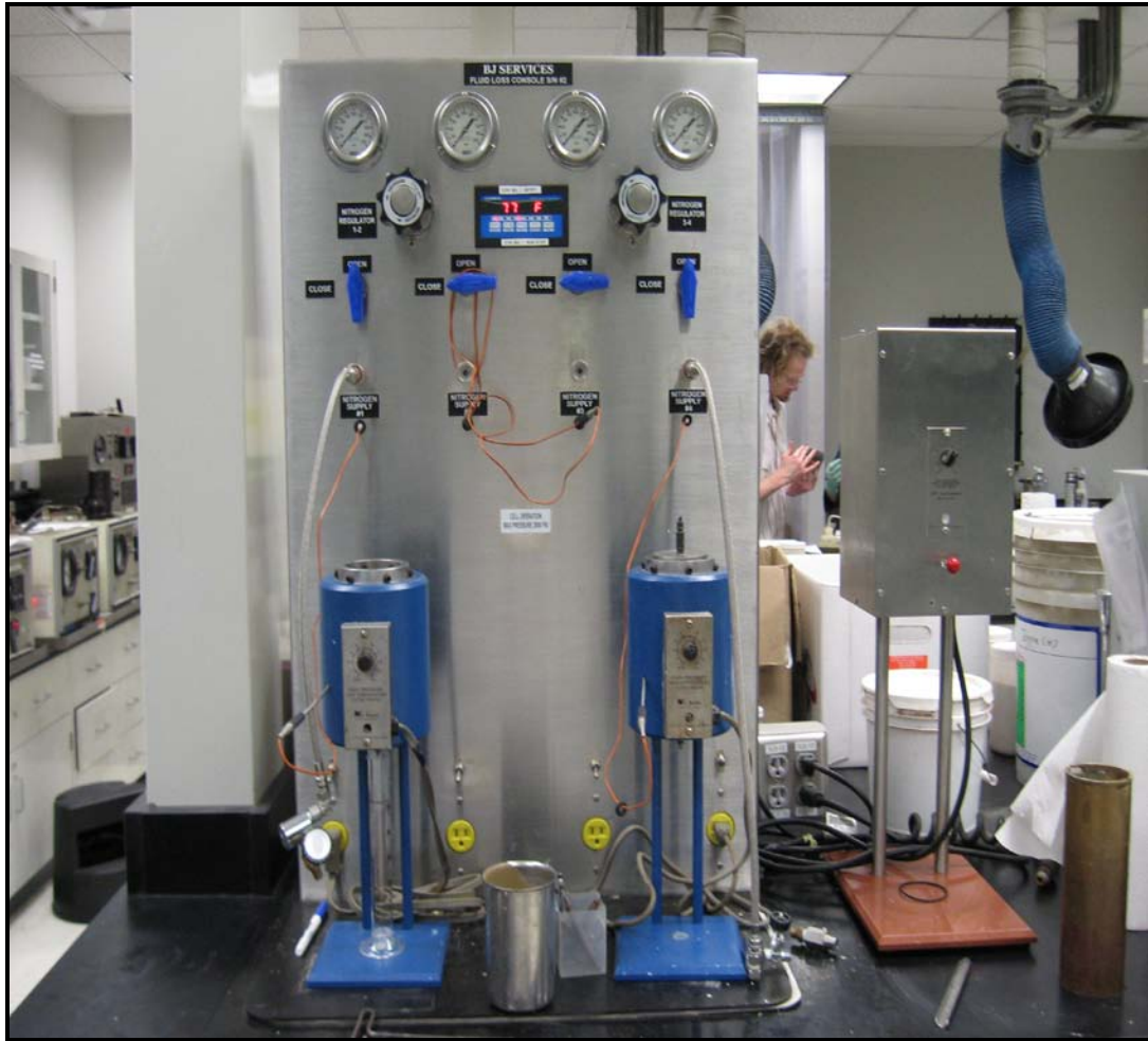
Figure 26: Stirred Fluid Loss Tester at BJ Services, Tomball, TX
