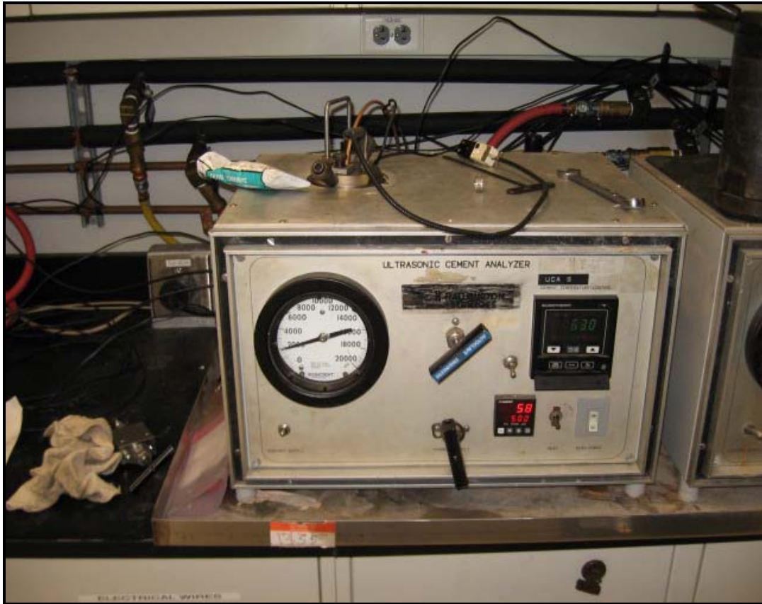
Figure 20: Ultrasonic Cement Analyzer for Compressive Strength Testing
