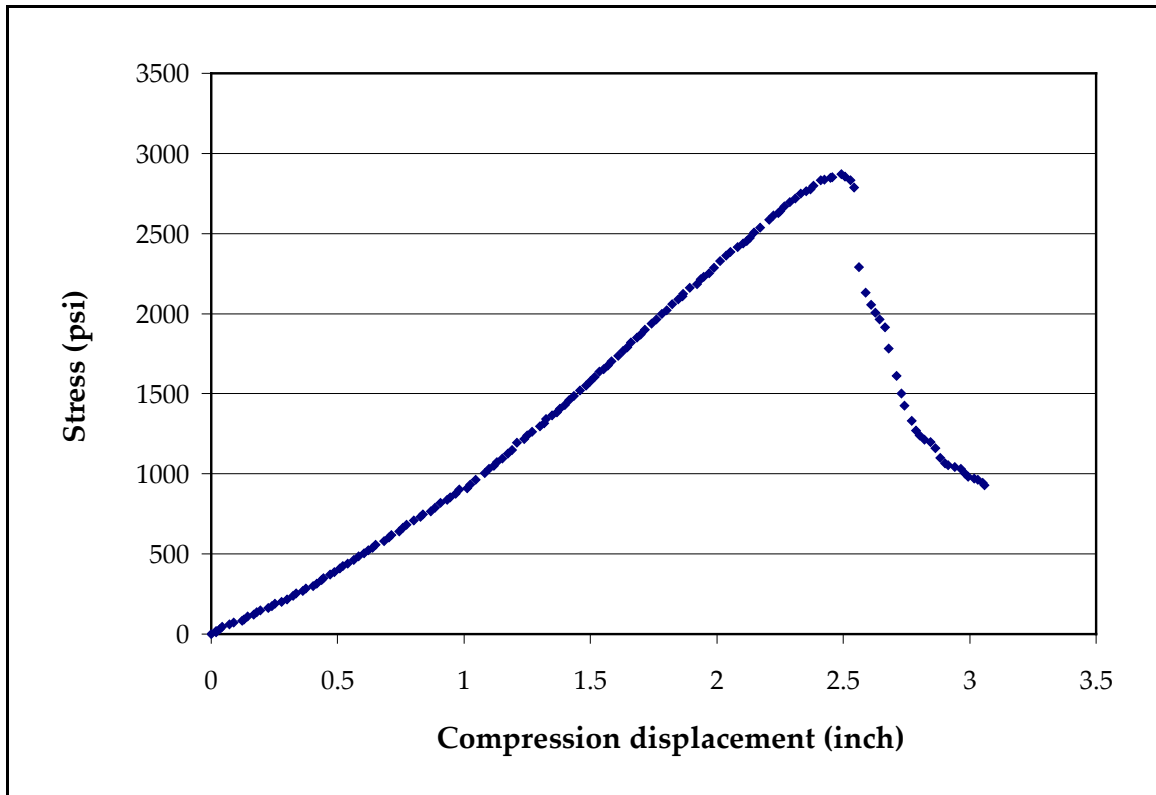
Figure 42: Compression Testing Data for Sample Ceramicrete Formulation #1 Without 5% Contamination by Dry California Portland Cement "G" Grade at Room Temperature (Load rate = 47.6 lbs/sec).
