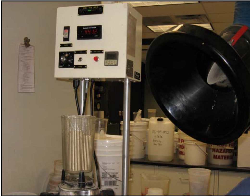
Figure 15: Blender Used to Mix 95% Ceramicrete and 5% Dry California Portland Cement "G" Grade.
