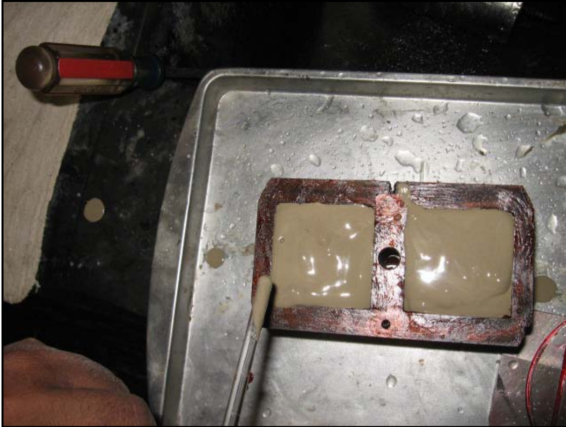
Figure 23: 2" x 2" x 2" Molds with Mixture of Ceramicrete Slurry and 5% California Portland Cement "G" Grade for Compressive Strength Testing.
