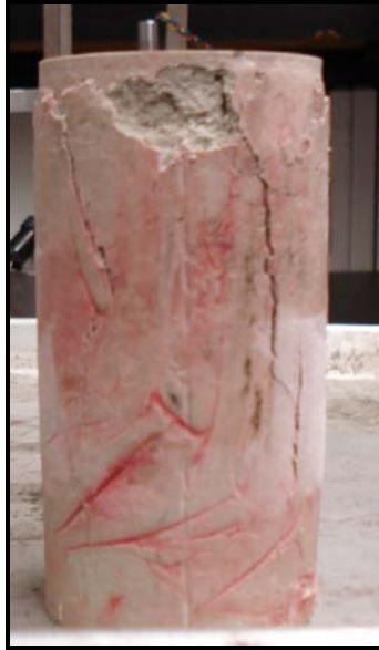
Figure 39: Ceramicrete Compression Samples (Post-Fracturing)
