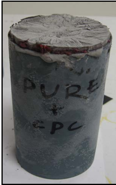
Figure 35: Expansion of Base Ceramicrete Sample with Contamination by 5% Dry California Portland Cement "G" Grade at 32 Degrees F After 24 hrs
