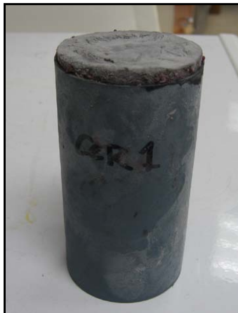
Figure 36: Expansion of Sample Ceramicrete Formulation #1 at 32 Degrees F After 24 hrs
