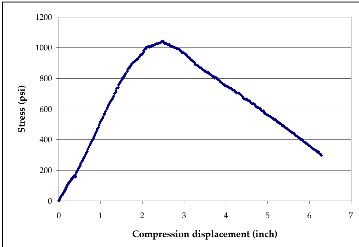
Figure 45: Compression Testing Data for Sample Ceramicrete Formulation #2 With 5% Contamination by Dry California Portland Cement “G” Grade at Room Temperature (Load rate = 18.23 lbs/sec)
