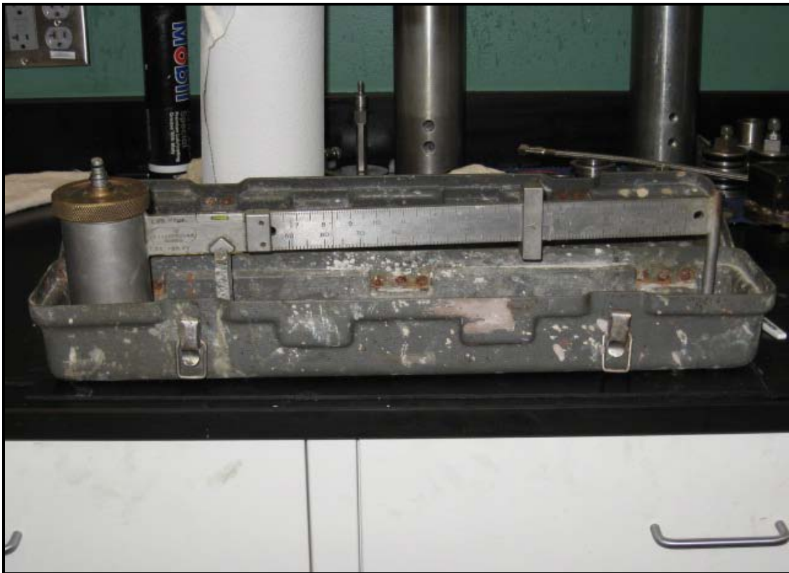
Figure 19: Halliburton Tru-Wate™ Pressurized Fluid Density Scale
