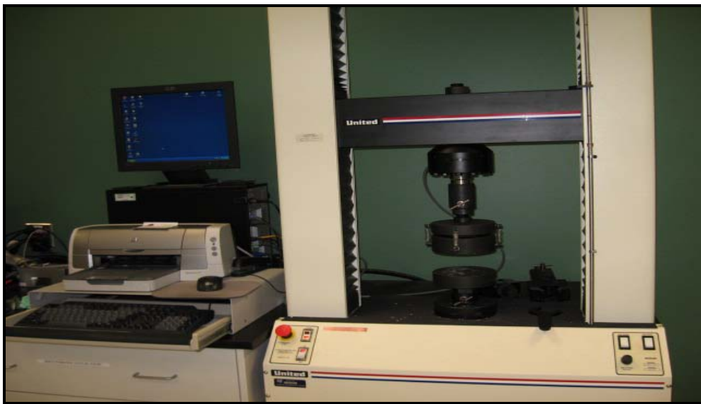
Figure 25: Instrument to Measure Compressive Strength of 2" x 2" x 2" Cubes at the R & D Center, BJ Services, Tomball, TX
