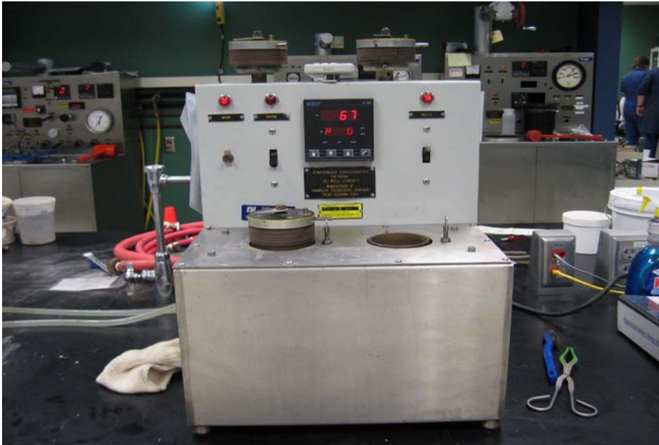
Figure 28: Atmospheric Consistometer for Conditioning Cement Slurry.
