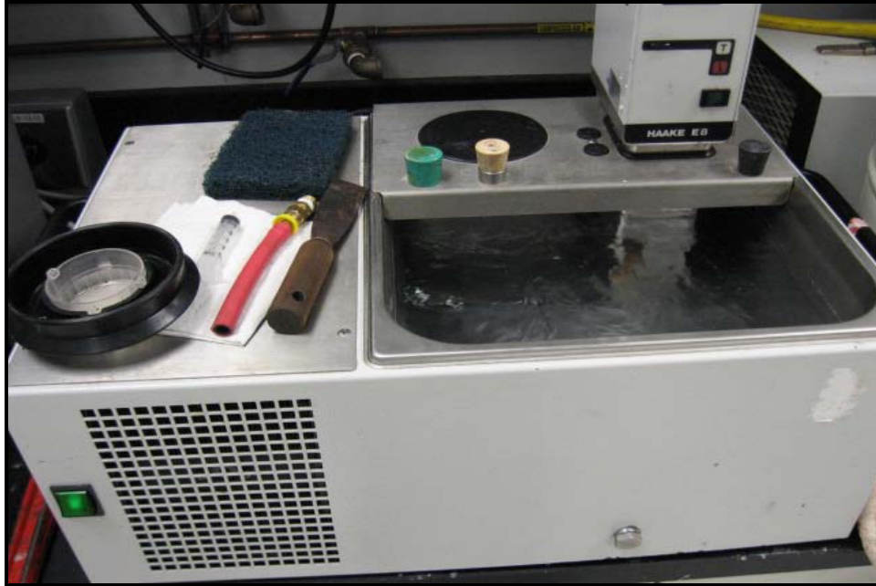
Figure 24: Model 200 HTHP Curing Chamber to Prepare Cement Specimens for Compressive Strength Testing
