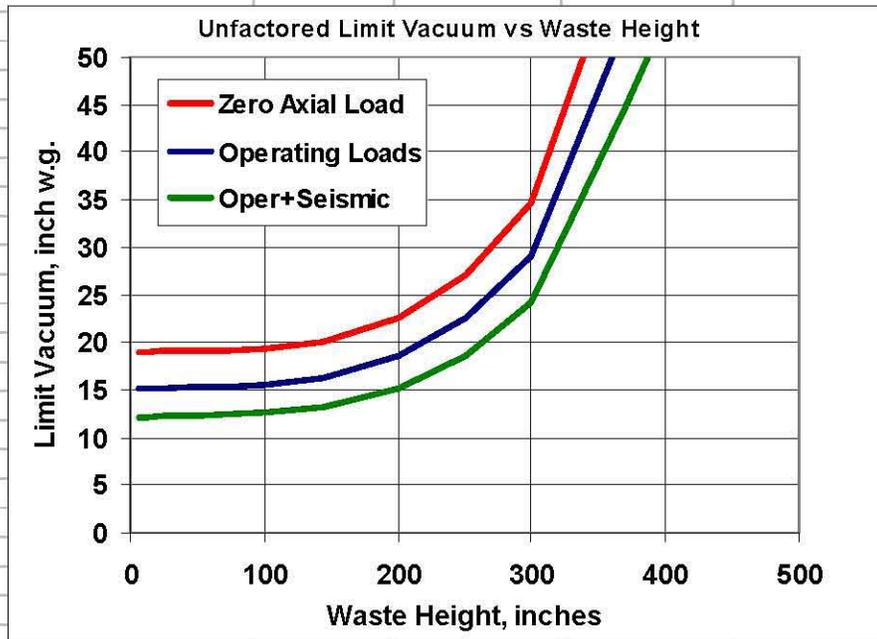
Figure F-2. Unfactored Buckling Limit Vacuum as a Function of Waste Height for the AY and AZ DSTs (Note: To calculate the factored vacuum limits, one must divide by the appropriate safety factors in the table of Section 2.1.)
