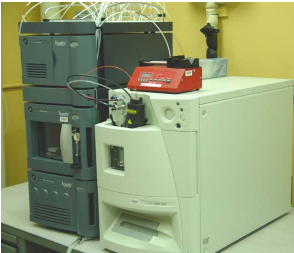
Figure 3. UPLC/MS Instrument Installed in WRI Laboratory
