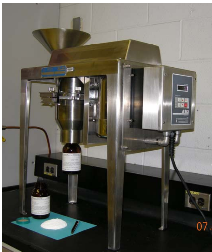
Figure 14. Comil 197 Lab Model Grinder purchased from Quadro.
