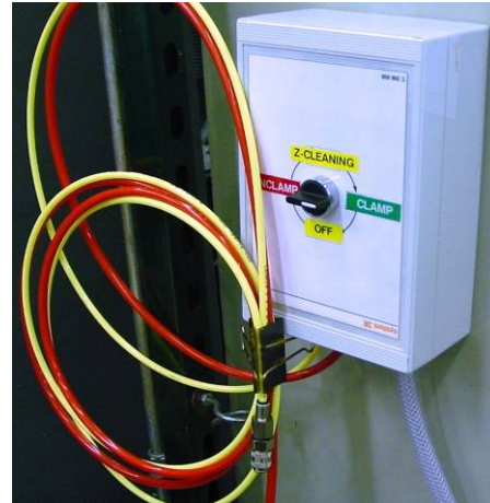
Pallet System Installed on Monarch VMC-75B Pneumatic Clamping Control System
