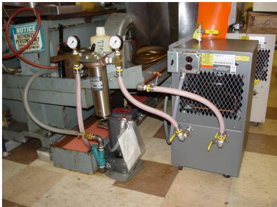
Figure 7. Typical Installation of a Chiller on a Lathe
