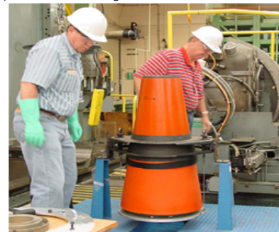
suction fabricator Body Sections for body is seated on a special blue fixture borrowed from Pantex. The orange neoprene covers on the body protect the surface.
