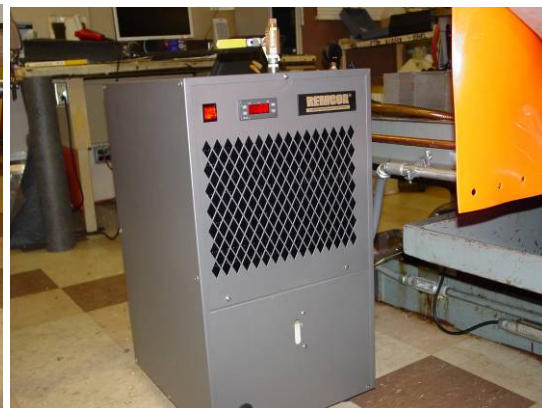
Figure 7. Typical Installation of a Chiller on a Lathe
