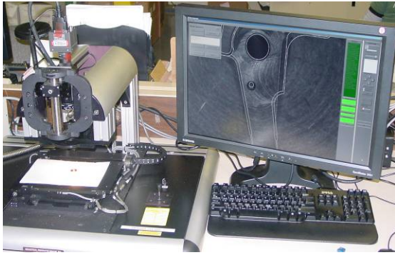
VOC With Part Being Inspected on White Paper Video Image of Part With Overlaid Tolerance Bands
