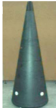
The black epoxy heat shield covering the body cannot be touched by bare skin, requiring the work to be done with extra care.
