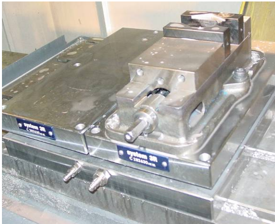
Pallet System Installed on Monarch VMC-75B Pneumatic Clamping Control System
