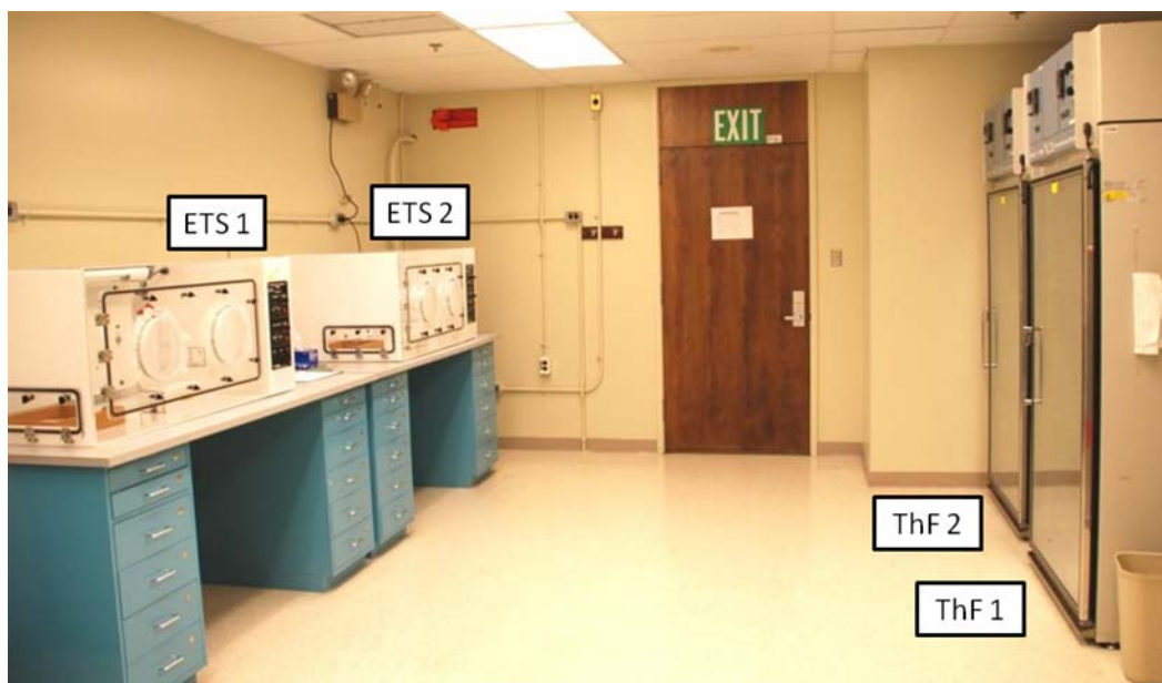
Fig. 3. The four environmental chambers at LLNL used for particle storage and conditioning
