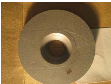
Picture 2: Cleaned coupon from SDA-OUT after exposure to CaCl 2 -enriched flue gas. Notice the bullet-shaped pattern across the face. "Bullet" points downstream of flow. Dark spot is a stain on the metal surface – cause yet unknown.
