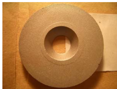
Picture 3: Cleaned coupon from SDA Roof after exposure to CaCl 2 -enriched flue gas. Notice the raised area around the center chamfer caused by exposure protection from the 0.25" Teflon spacer.
