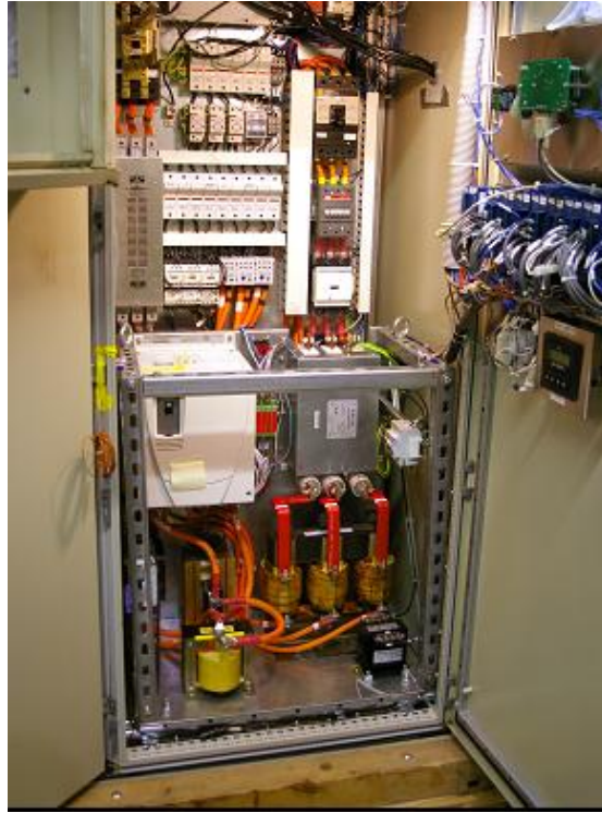
Figure 3.2-1: DC Motor drive Test Setup
