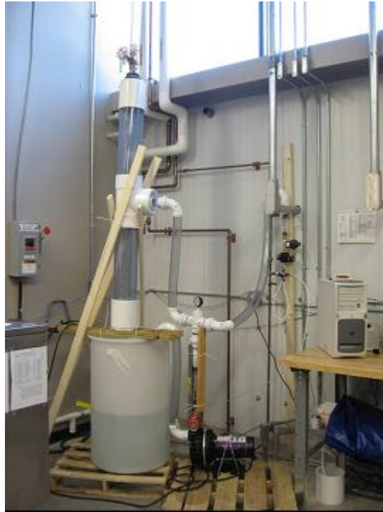
Figure 3.5-1: Full Scale Oxygen Separator Mock-up
