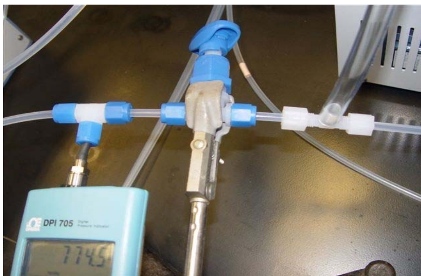
Figure 4. Back Pressure Experiment Valve
