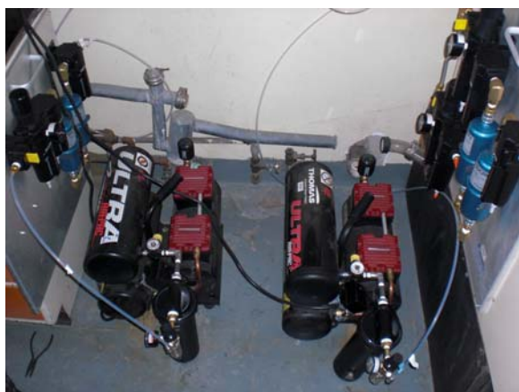
Figure 3. Oil-free Air Compressors with Tekran Air Purification Manifolds
