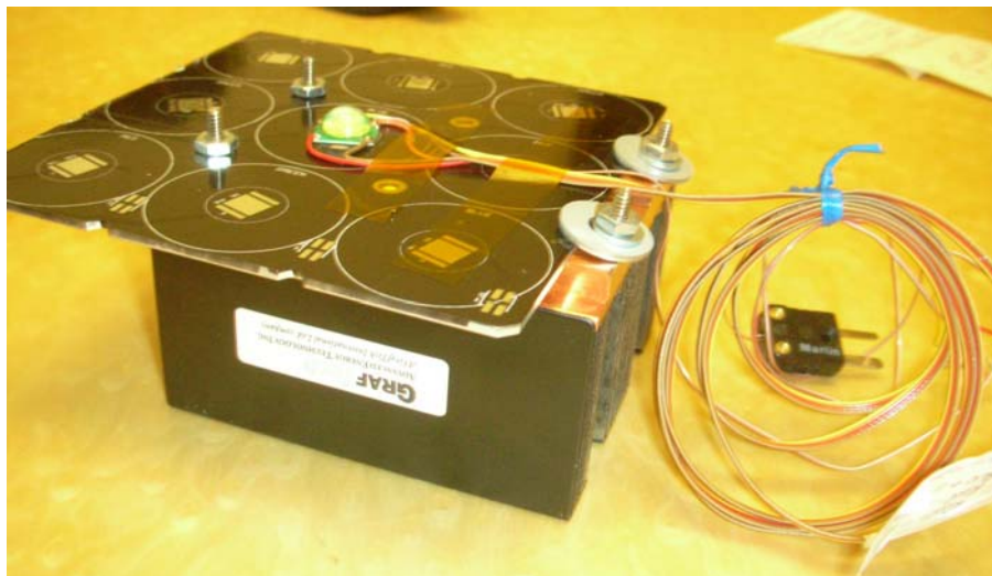
Figure 24. Test configuration for the LED engine performance test. The LED package was mounted to a metal-core board from another prototype fixture and tested in situ for light output.
