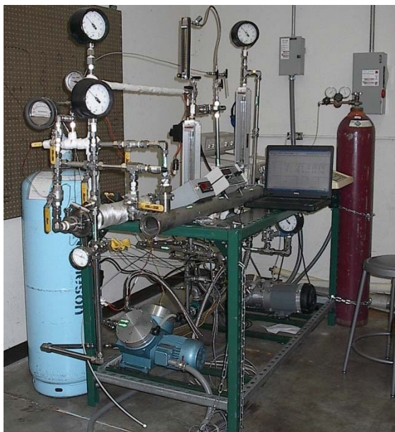
Figure 7. Mixed-gas bench-scale module test system.
