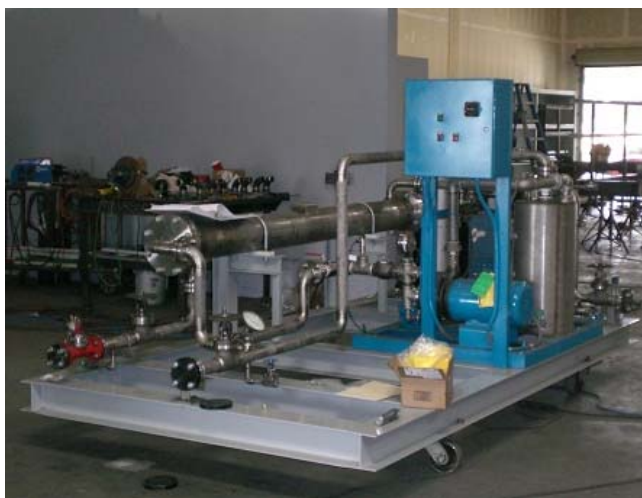
Figure 14. Photograph of an MTR membrane test skid for enriching CO 2 from natural gas-fired flue gas. This unit has been delivered to APS' Red Hawk natural gas-fired power plant, just west of Phoenix, AZ.
