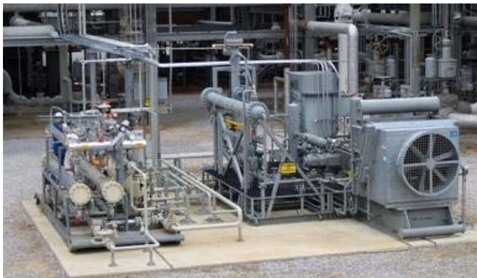
Figure 13. A picture of an MTR membrane test skid for treating natural gas. This unit was installed at BP's Pascagoula, Louisiana gas processing plant.
