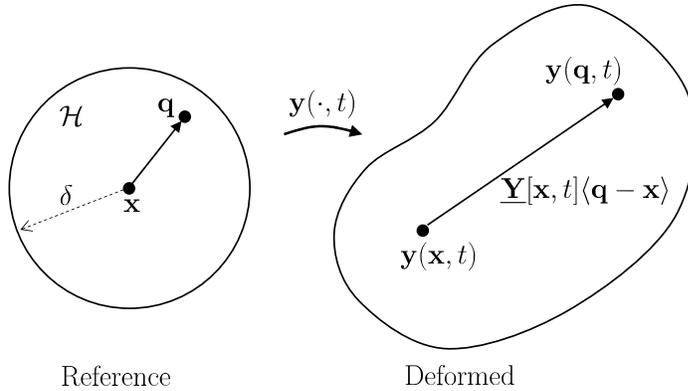
**Figure 1.** The deformation state  $\underline{\mathbf{Y}}$  maps a bond  $\mathbf{q} - \mathbf{x}$  into its deformed image.
