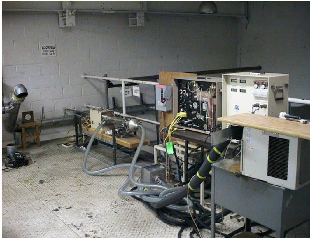
Figure 6. Particulate Sampling and Measurement System
