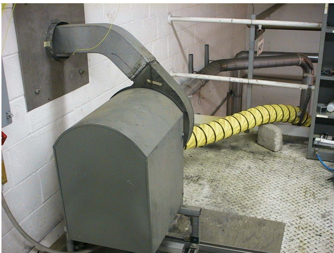
Figure 5. Sampling Stack With Induced Draft Fan Shown at Mezzanine
