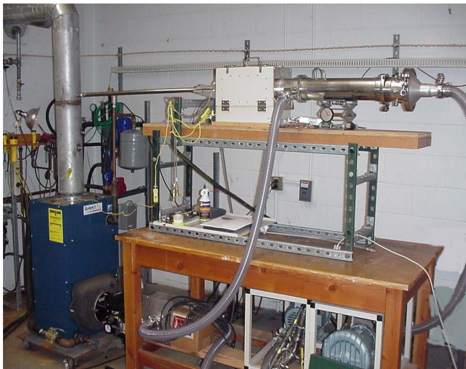
Figure 7. Boiler and PM 2.5 Sampling for Filter Temperature Tests
