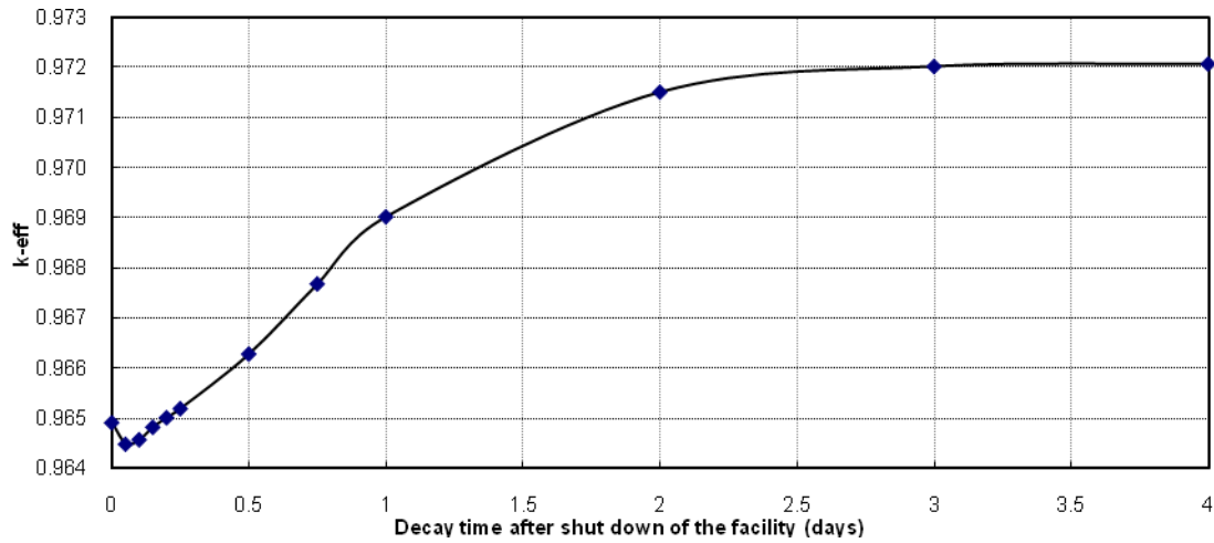
Figure 17. k-eff as a function time during the shutdown time after the first burnup stage
