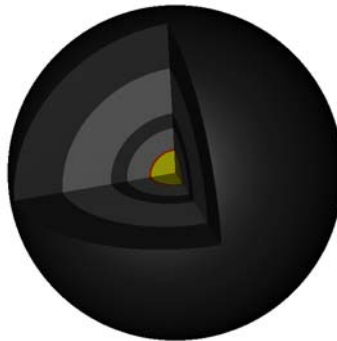
Figure 3. Cutaway schematic of one example of Phantom 3: Nested Spherical Shells. DU is yellow, tungsten is light gray and lead is black. Sphere and shell properties are given in Table 3.
