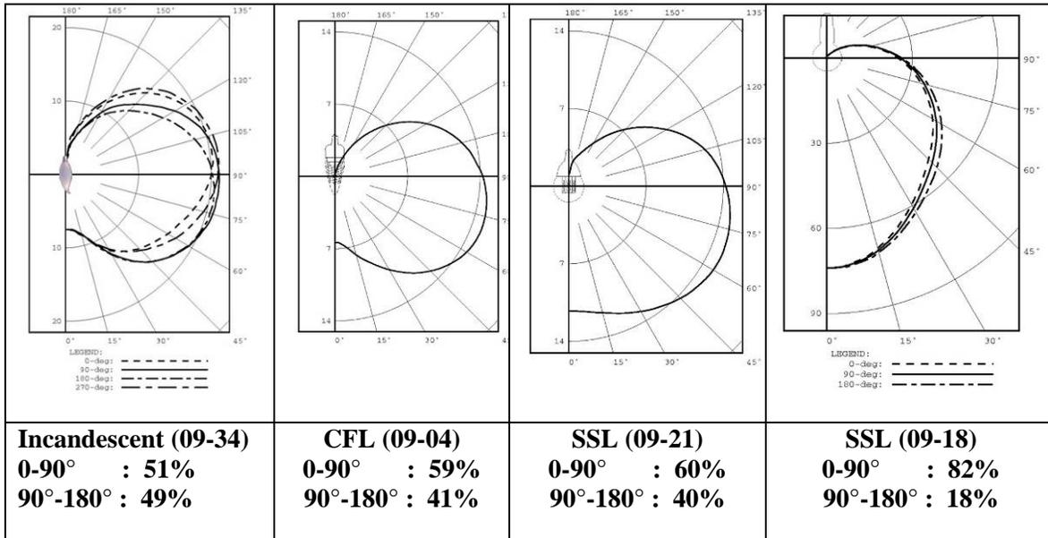
**Figure 5.** Comparison of Light Distribution of SSL Omni-directional Replacement Lamps with Incandescent and CFL
