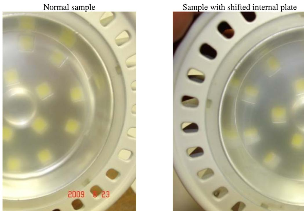
**Figure 9.** Example of Unexpected SSL Failure Mode
