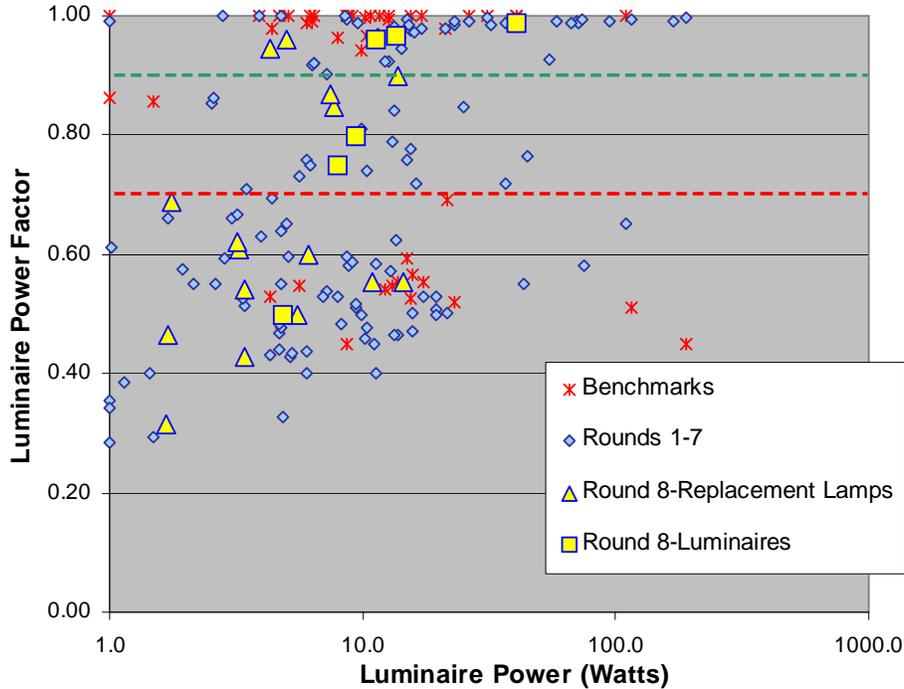
**Figure 8.** Power Factor Versus Wattage for CALiPER-tested SSL Luminaires and Replacement Lamps
