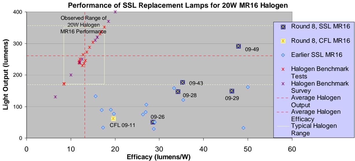
Benchmark values are based on CALiPER benchmark tests, surveyed ratings, and averaged manufacturer ratings for 20W MR16 halogen lamps. Values are based on initial output, not average life-time output.
