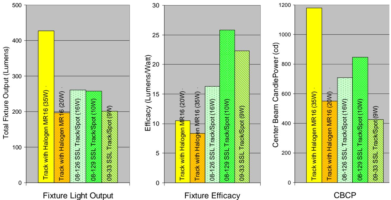
**Figure 6.** Comparison of SSL Track Lights to Track Light Fixtures Using 35W and 20W Halogen MR16 Lamps Based on 120VAC input, assuming overall fixture efficiency (including optical and driver/transformer losses) of 0.75 for halogen-based track lights, using average surveyed manufacturer ratings for MR16 halogen and HIR lamps.
