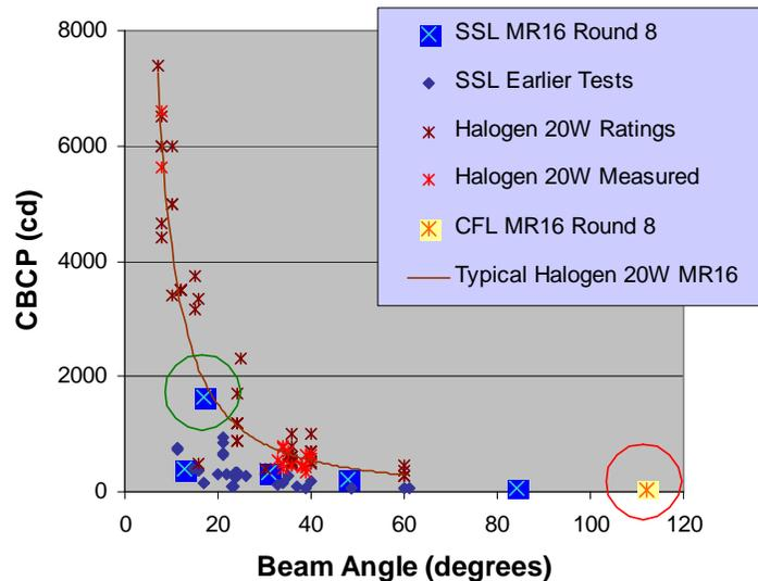
**Figure 3.** CBCP Versus Beam Angle for SSL, CFL and Halogen MR16 Lamps
