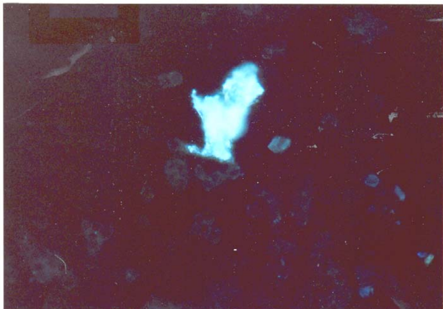
Figure 36. The same field as in Figure 37 but taken under UV light showing that the small particles are only weakly fluorescent while the less common ones fluorescence intently.
