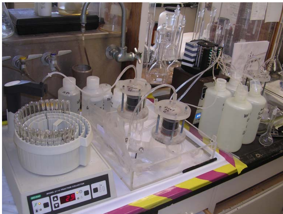
Figure 1. Experimental set-up for the grout columns during the tritium pulse test using a fraction collector.
