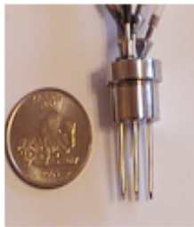
Prototype cooling device, including seven needle-shaped cooling probes and temperature sensor, optimized to cool brain tissue in order to stop seizures.
