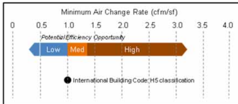
Figure 5. Benchmarks area-based minimum ventilation rates
