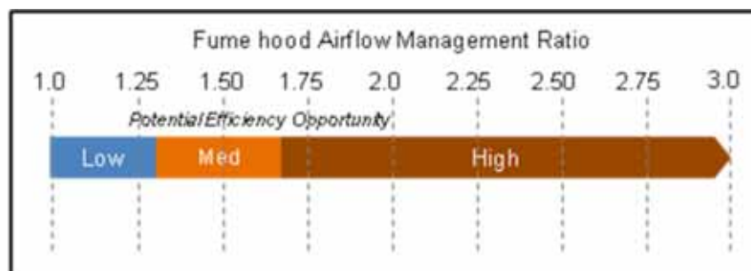
Figure 11. Benchmarks for fume hood airflow management ratio
