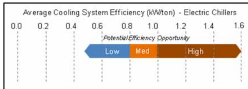
Figure 15. Benchmarks for overall cooling system efficiency for electric chillers
