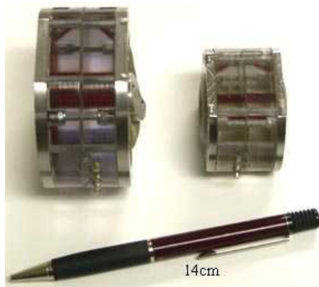
High Resolution Seismometer Insensitive to Extremely Strong Magnetic Fields
