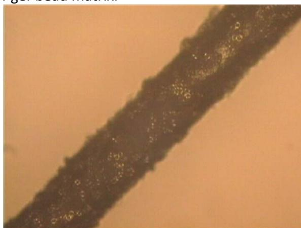
**Figure 21 Sol-gel-bead matrix cured within a closed microchamber.**
