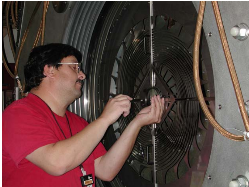
Figure 37. Installation of a primary coil into the pulsed power driver system.
