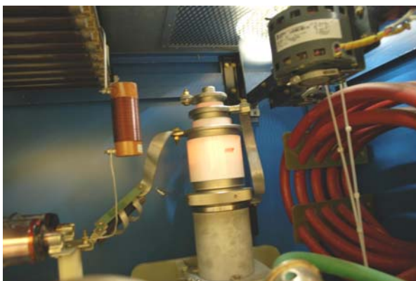
Figure 2. Vacuum tube in the rf generator during the test run.
