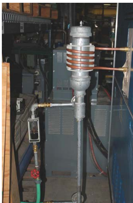
Figure 3 Test load coil for rf generator.
