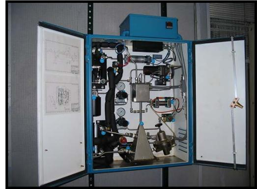
Figure A-2. Pierburg fuel metering system
