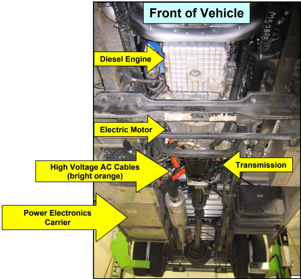
Figure 4. Eaton hybrid system components on UPS undercarriage
