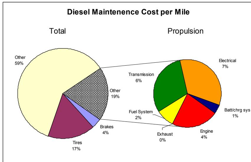
**Figure 13. Propulsion maintenance cost per mile (diesels)**
