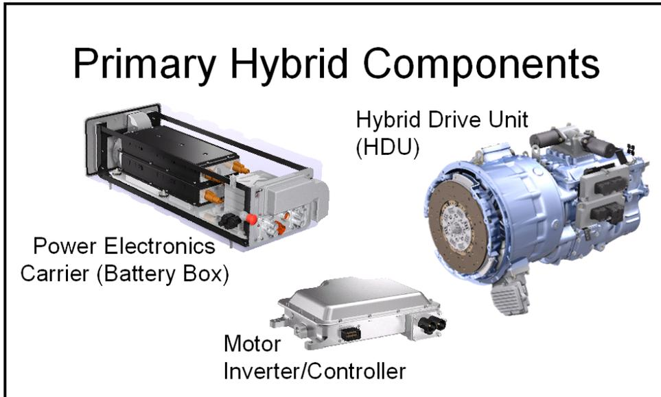
**Figure 3. Eaton hybrid system components**
