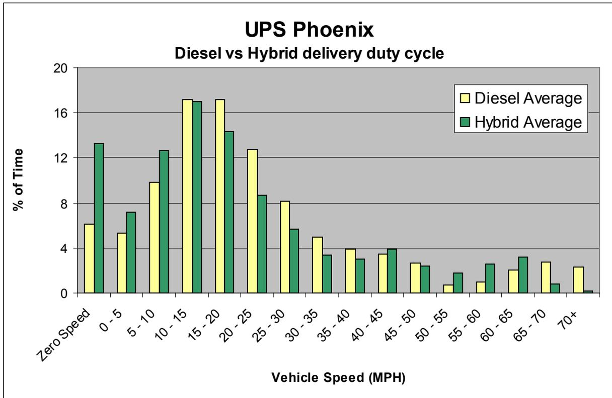
**Figure 8. Hybrid and diesel duty cycle breakdown**
