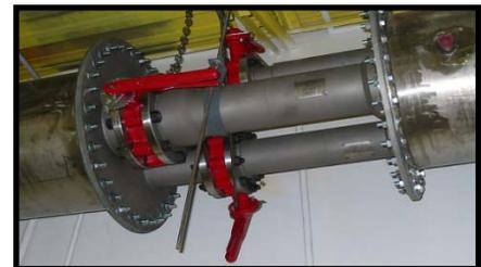
Figure A-3. Venturi nozzles
