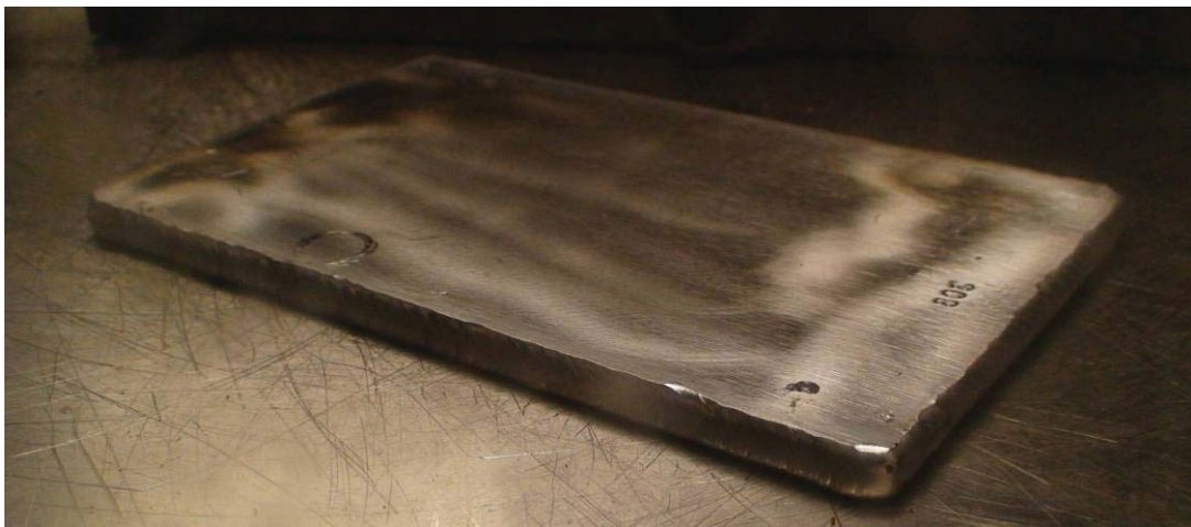
Figure 8. Welded rolling assembly ready for hot rolling process.
