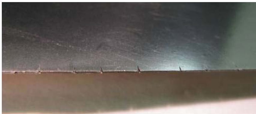
Figure 14. Photo showing edge cracking of foil.
