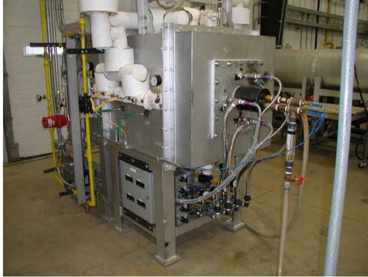
Figure 14. Laboratory DFI Furnace Installed at GTI (with Round Calorimeter Inserted)
