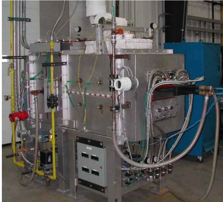
Figure 22. GTI's Laboratory DFI Furnace Reconfigured for Testing Flat Loads (with Flat Calorimeter Inserted)
