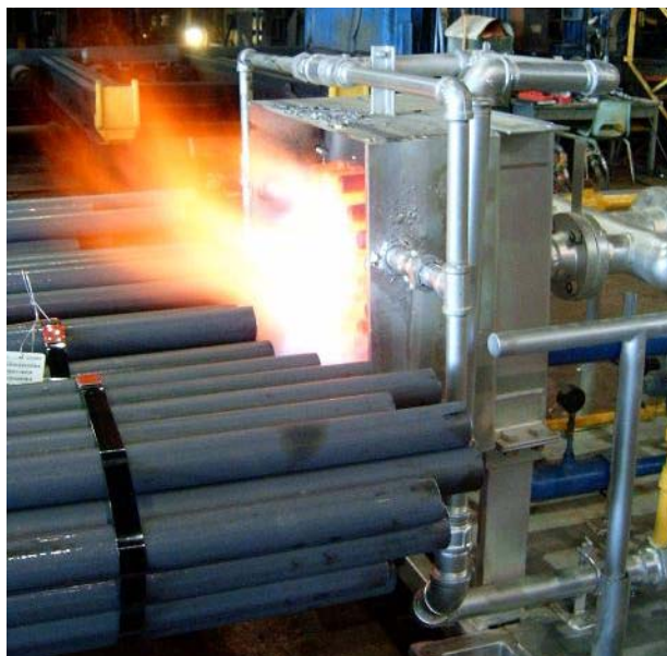
Figure 48. Portable DFI Heating Cart in Operation at REP
