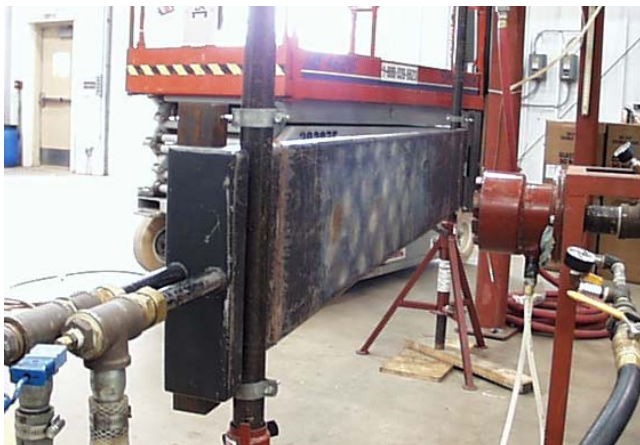
Figure 49. Side View of Setup for Testing Performance of Alternate Burner
