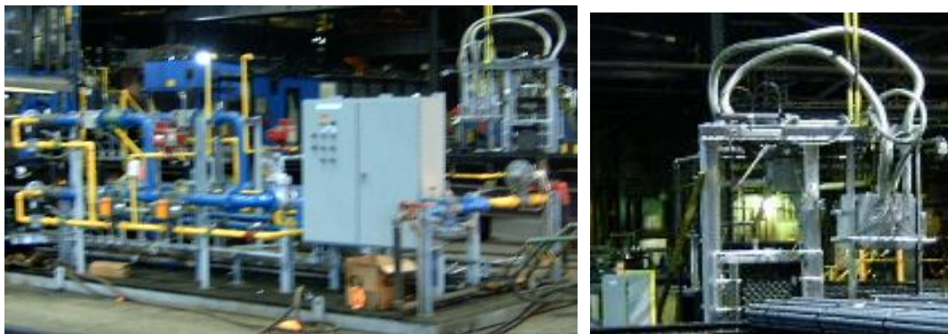
Figure 45. Flow Skid and Burner Stand Installed at REP
