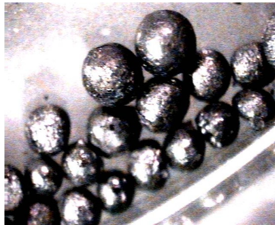
Figure 2. UC particles produced by the rotating electrode method.
