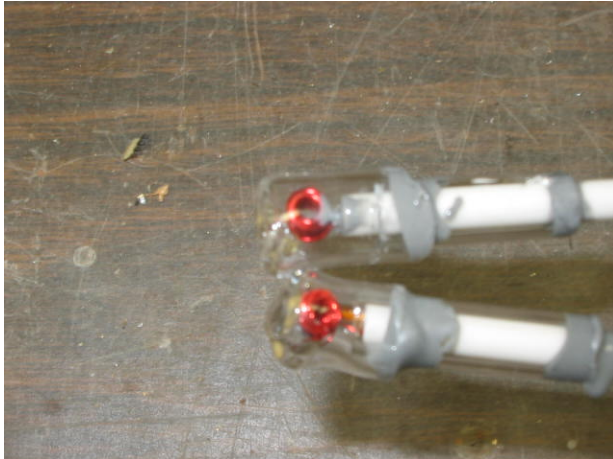
Figure 1. The emitter and receiver coils with Pyrex caps to protect them from the plasma. The JB Weld holds the Pyrex to the ceramic tube. Right: Circuit schematic for the emitter driver.
