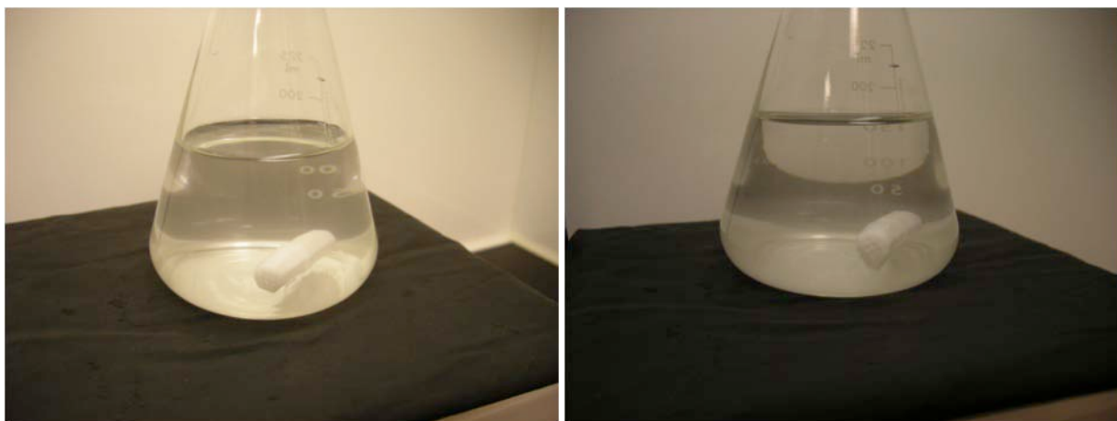
Figure 4b. Precipitation of magnesium hydroxide and silica by NaOH immediately after (left) the end of stirring, and only gradual clearing in progress 20 minutes later (right). The lingering haze of fine particulates may be more difficult to remove by sand bed filtration than is the alumino-silicate floc seen above in Fig. 4a.
