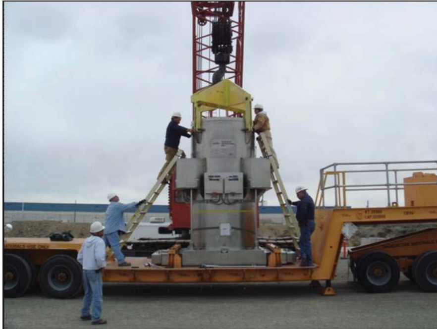
Figure 7. A 55-ton scrap cask used for transporting waste to the disposal facility.
