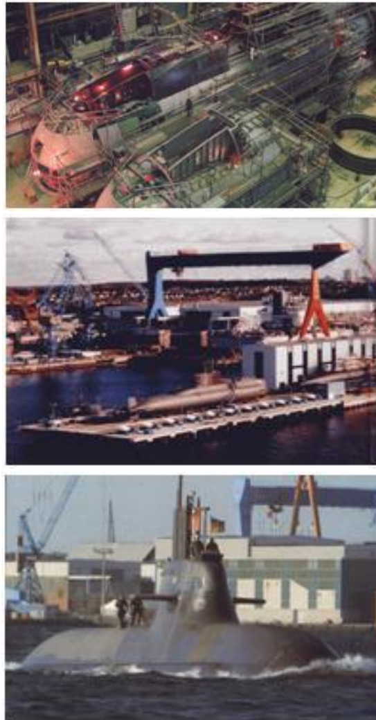
Figure B 1 – The left image shows the Class 212A fuel-cell powered submarine being constructed by HDW in Kiel, Germany. The center image shows the assembled submarine sitting in dry dock, and the right image shows the vessel after launch
