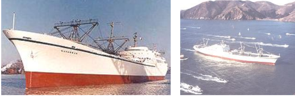
Figure A 1 – The commercial NS Savannah nuclear powered ship was built by New York Ship Building in Camden, New Jersey and had a 74 MW PWR built by Babcock & Wilcox (B&W) and sailed from 1970-79
