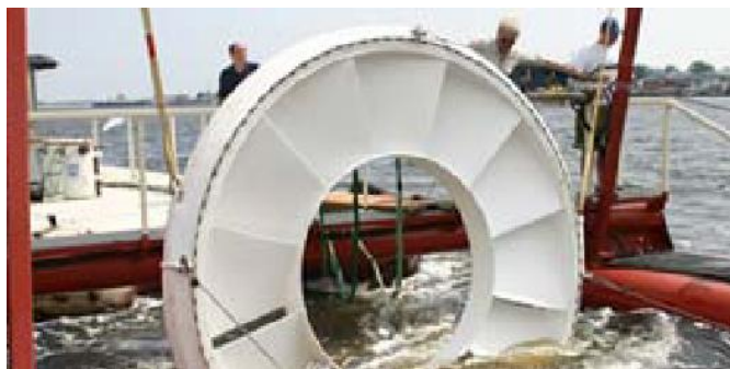
Figure E 1 – Advanced turbine for the conversion of deep ocean current to shaft energy
