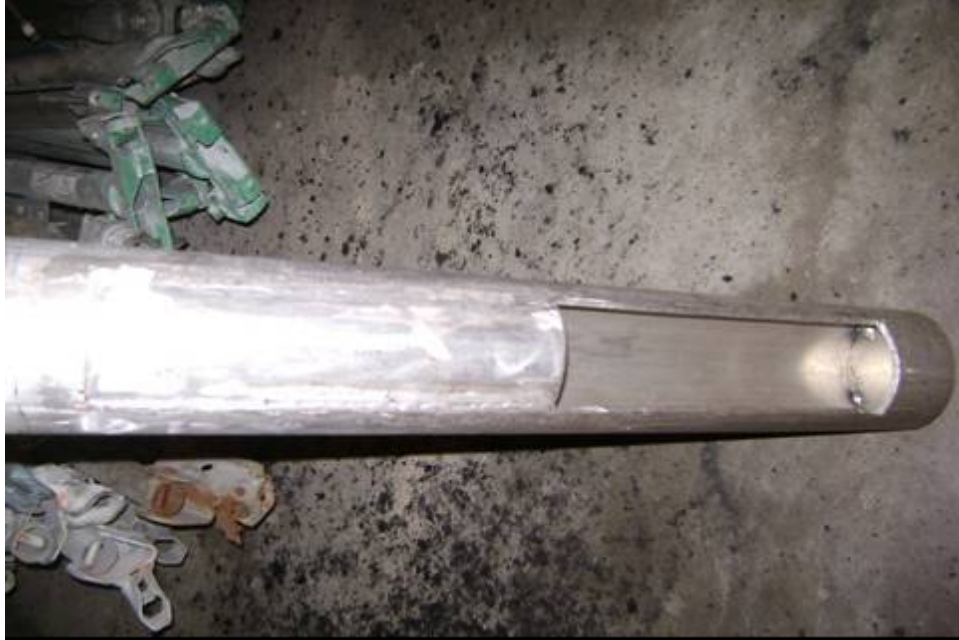
Figure 16: Coal Sampling Probe
