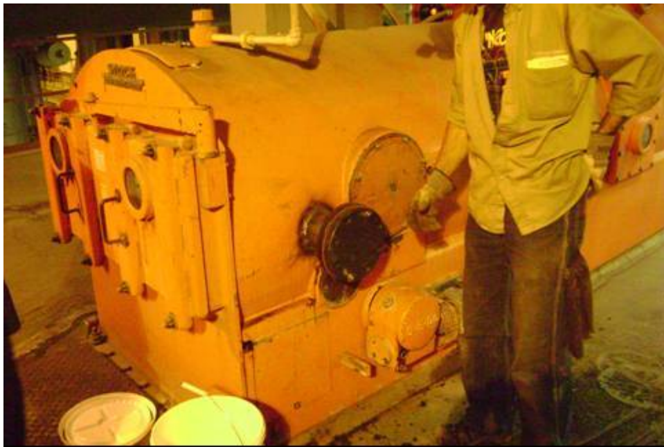
Figure 16: Coal Sampling Probe
