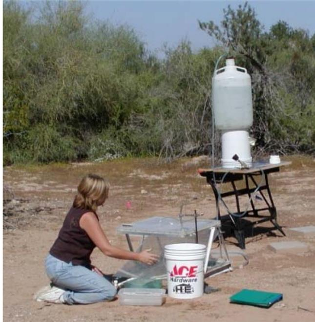
Figure 3. Photograph of portable rainfall simulator.
