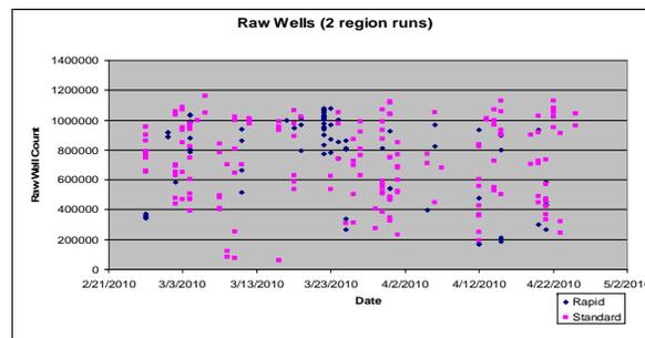
We discovered that robotic processing was not fully removing null beads and they were being loaded into PTPs and were producing runs with low numbers of raw wells as indicated in the chart above.
