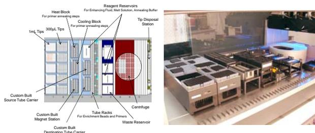
At present the enrichment robot can parallel process up to 8 samples, with changes to its program the deck layout will support up to 24 samples at a time. Program duration for a double enrichment run is 3.5-4 hours.
