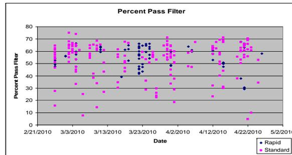
By examining run metrics over the same period we were able to determine that low total number of bases per region was not caused by an overall lower quality of beads coming out of emPCR. The chart above shows the percent of beads passing mixed/dot/tooshortquality/tooshort primer filters averaging between 55-70%.
