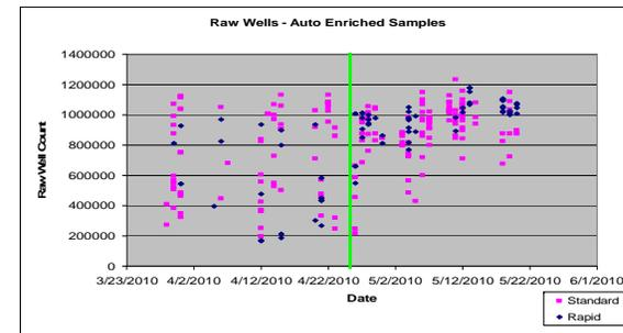
Beginning 4/26/2010 the JGI introduced an improved robotic pipetting method, incorporating additional null bead removals as well as enriching every sample twice using a single enrichment kit's worth of reagents. We saw a dramatic tightening in the range of raw well counts we were seeing in both our Rapid and Standard Library runs.
