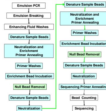
We made two changes to the robotic procedure as detailed in the process flowchart to the left.
