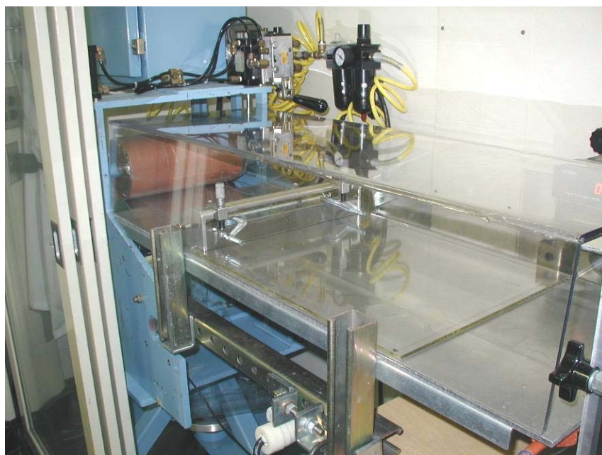
Figure 9. Casting of large films with new caster.
