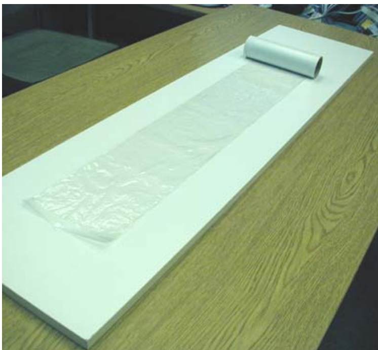
Figure 3. BisSF-BPSH (22k-14k) block copolymer films. The film appears to be void-free and uniform in thickness (10 \mu\text{m} ).
