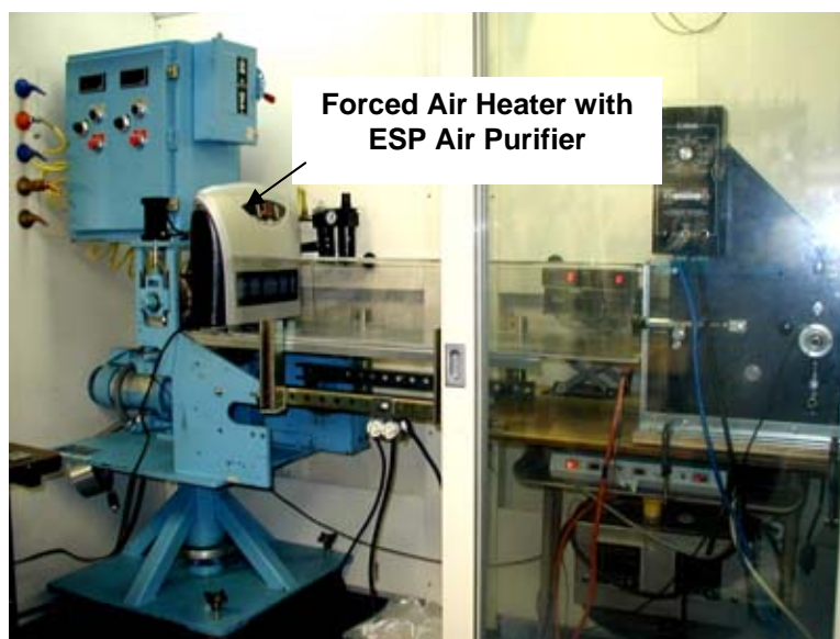
Figure 6. Picture showing the film casting system with new forced air heater with ESP air purifier.
