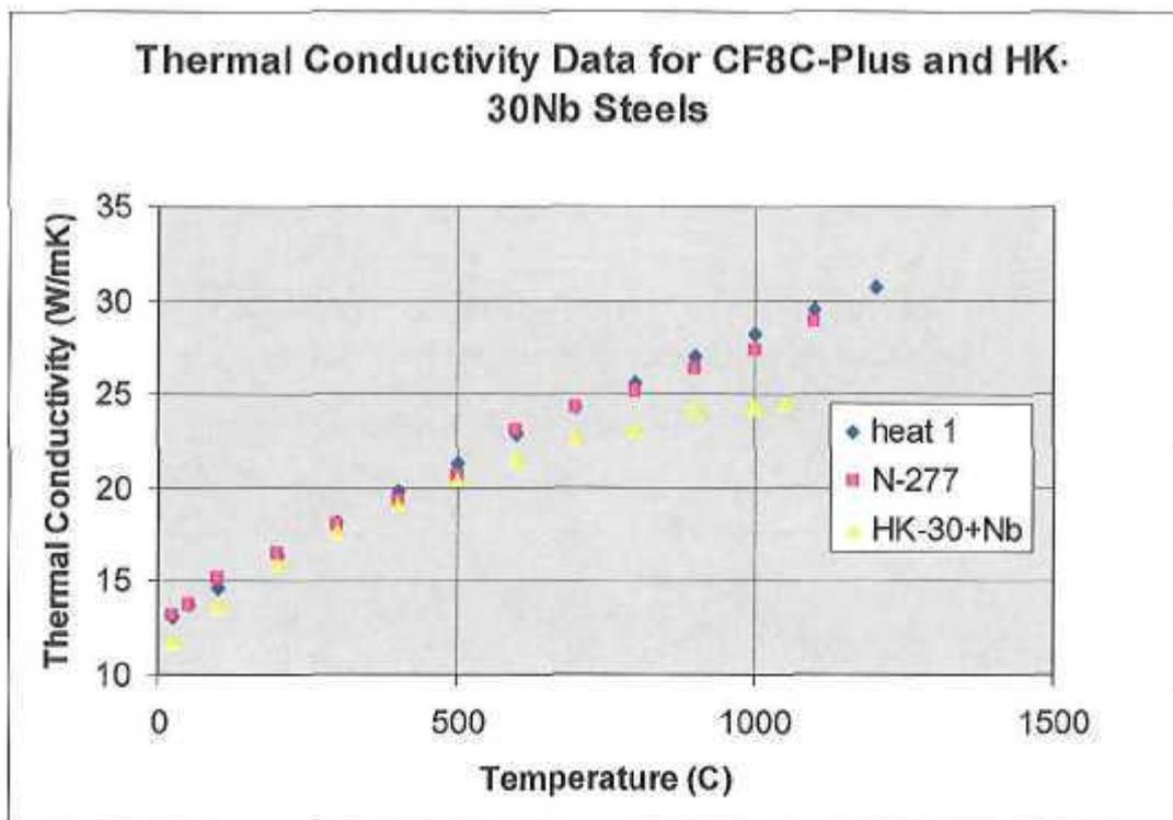
**Fig. 4** – Measurements of thermal conductivity CF8C-Plus and HK-30Nb cast austenitic stainless steels. Data for the N277 heat of CF8C-Plus steel and the HK-30Nb steel were provided by Honeywell for this CRADA project. Data for heat 1 of CF8C-Plus steel was provided to ORNL previously by Caterpillar.
