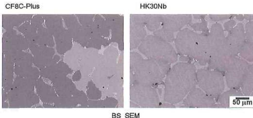
**Fig. 5** – Back-scattered scanning electron microscope (BS SEM) images of the microstructures of as-cast CF8C-Plus and HK-30Nb stainless steels. Both have equiaxed dendritic grain structures, with colonies of interdendritic precipitation, which are mainly NbC in the CF8C-Plus steel, and mixtures of NbC and Cr-rich  $M_{23}C_6$  in the HK-30Nb steel.
