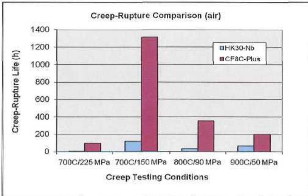
**Fig. 7** – Comparison of creep-rupture lives of as-cast CF8C-Plus and HK-30Nb steels for several different creep temperature and stress conditions. CF8C-Plus steel has more creep-resistance than HK-30Nb at each of these creep-rupture conditions.
