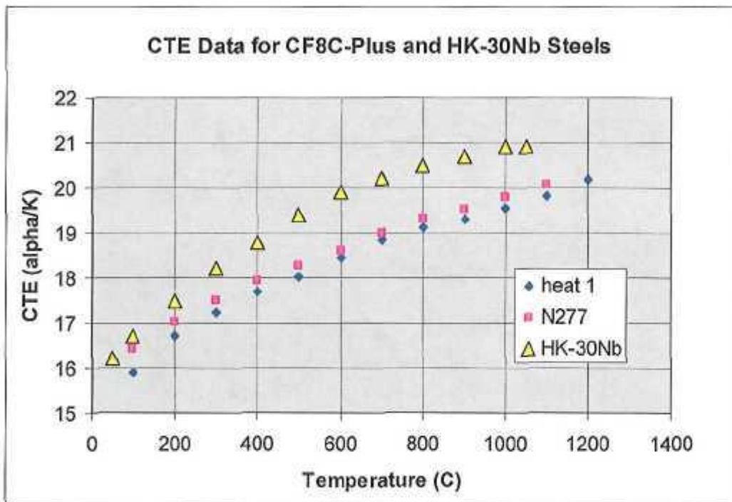
**Fig. 3** – Measurement of coefficient of thermal expansion (CTE) for CF8C-Plus and HK-30Nb cast austenitic stainless steels. Data for the N277 heat of CF8C-Plus steel and the HK-30Nb steel were provided by Honeywell for this CRADA project. Data for heat 1 of CF8C-Plus steel was provided to ORNL previously by Caterpillar.
