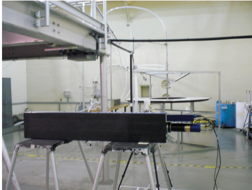
**Figure 4.1.** The Symetrica detector positioned for gamma insensitivity testing with the  $^{60}\text{Co}$  source in the background, the detector in the foreground and the neutron source in between.
