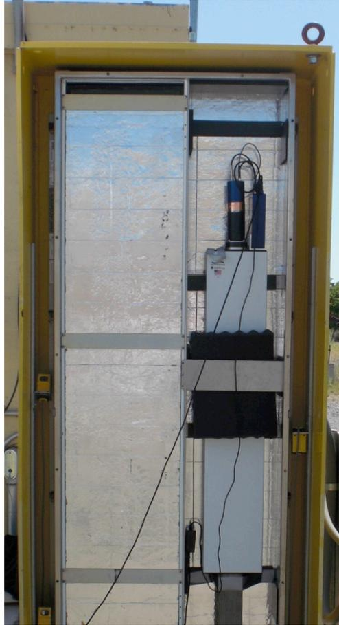
**Figure 3.2: Symetrica detector mounted inside the SAIC RSP for testing.**
