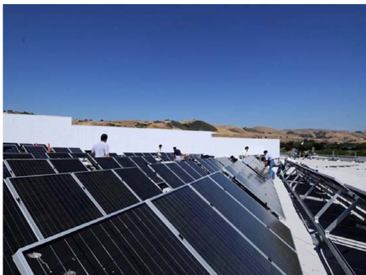
Figure 16. A view of SoloPower's rooftop testing facility with CIGS modules manufactured by SoloPower's electrodeposition-based technology. Photo credit: SoloPower
