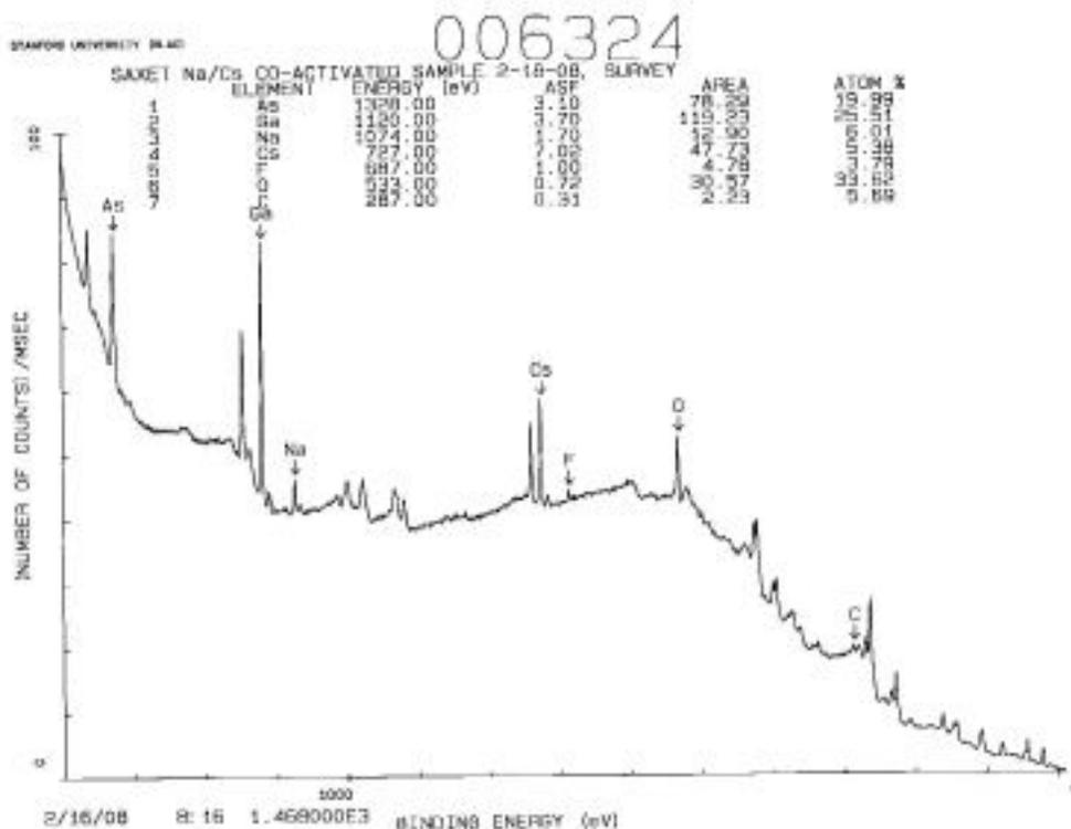
Figure 22. XPS survey spectrum of Na + Cs activated GaAs.
