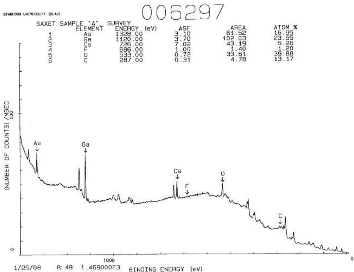
Figure 19. XPS survey spectrum of sample A, Cs only activated GaAs. The x-ray source was Al  $K_{\alpha}$ . The sample was activated and tested at Saxet then sent to SLAC for XPS work.
