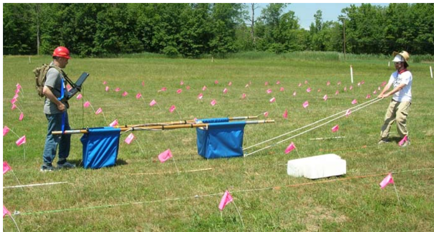
Figure 4. LBNL hand-held UXO discriminator at APG.
