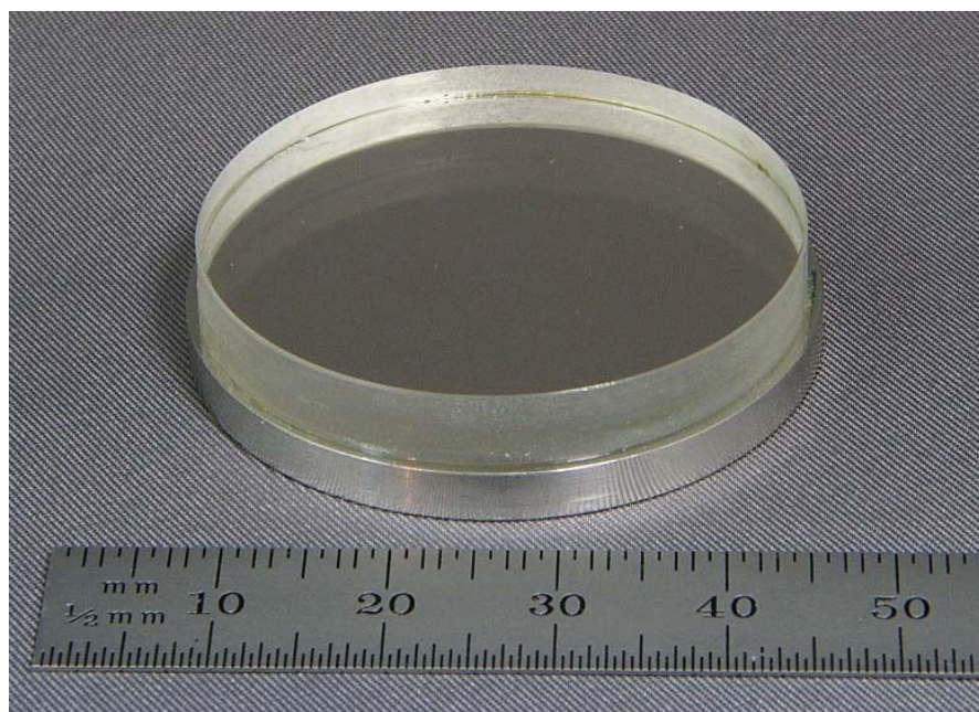
Figure 4. Typical sample with 2 mm thick tin and 3 mm thick lithium fluoride window
