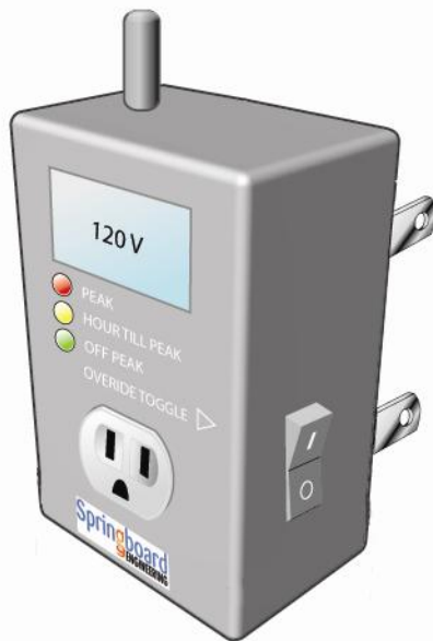
Figure 21: Concept Wireless Load Monitor and Control Device with Integral Customer Override Switch
