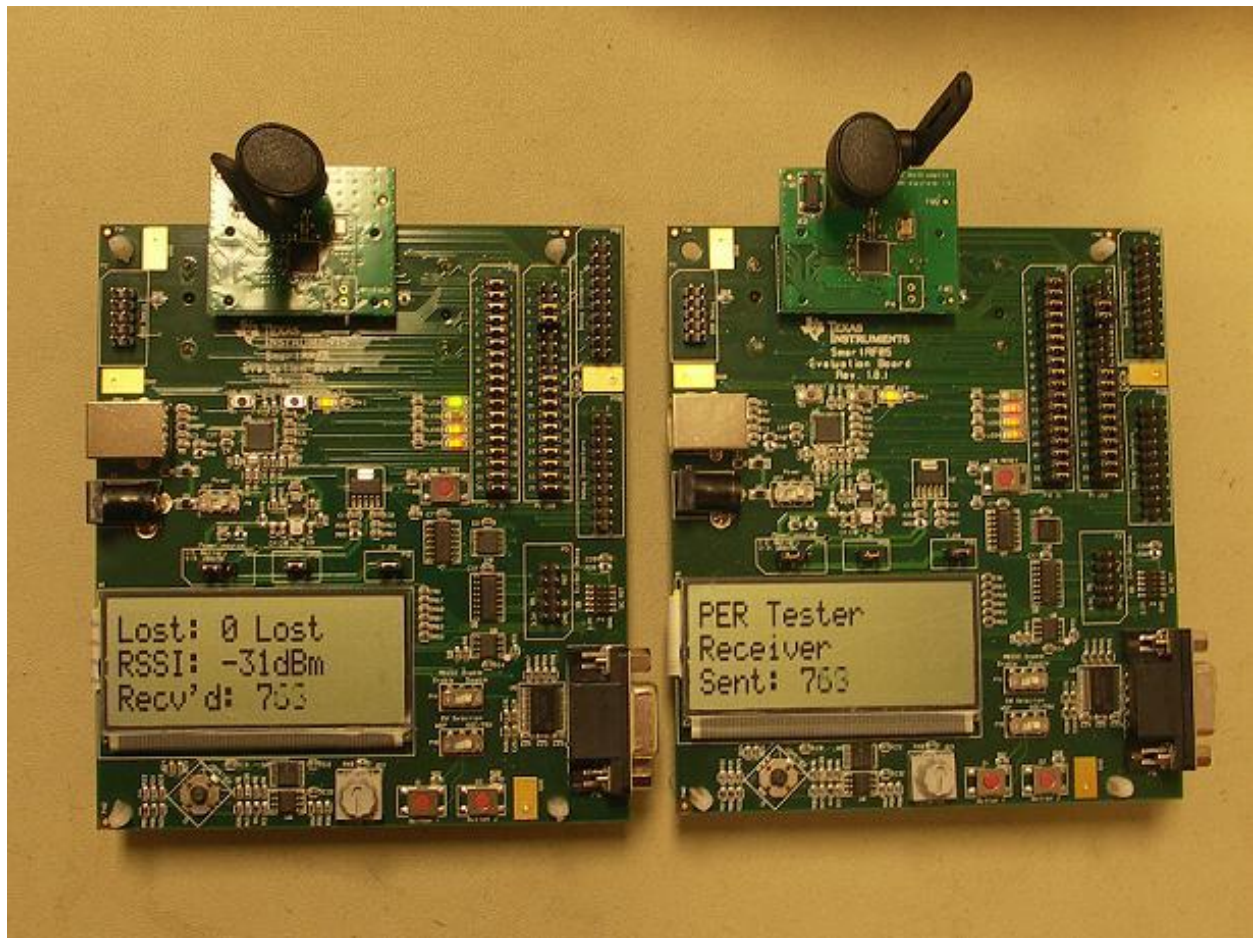
Figure 1 – Texas Instruments CC2530 Wireless Evaluation Kit
