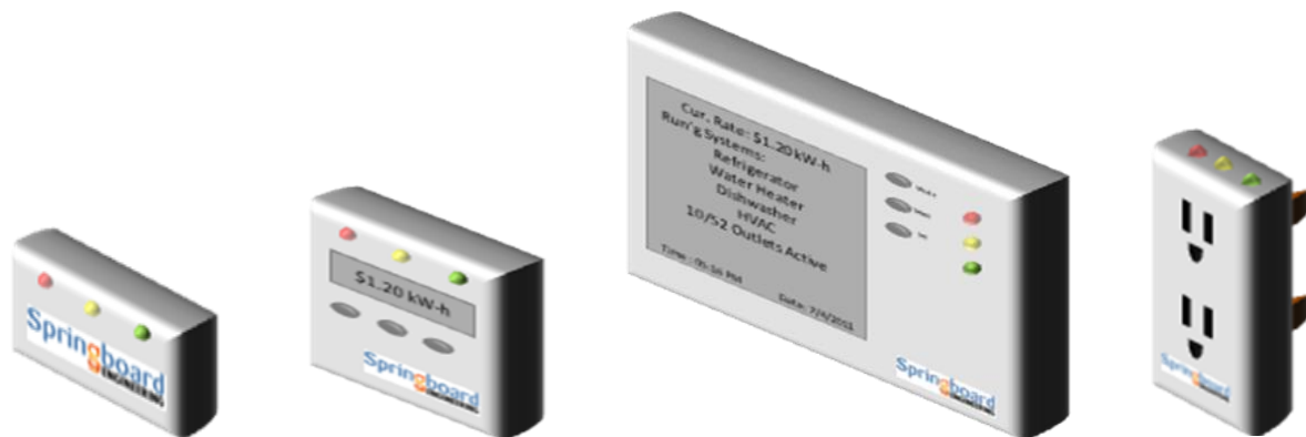
Figure 19: Concept Wireless Time-aware Devices that Communicate with the AMI and Indicate Cost Level to the Customer
